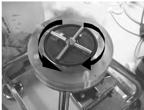
FIGURE 2.4 Oscillating spider distribution system.
