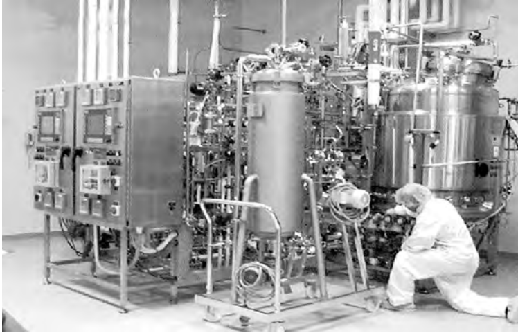
FIGURE 18.6 1000 L perfusion bioreactor and spin filter for manufacturing of infliximab at the Malvern manufacturing site.
