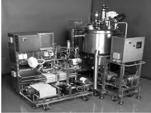
FIGURE 10.24 Ultrafiltration process skid.
