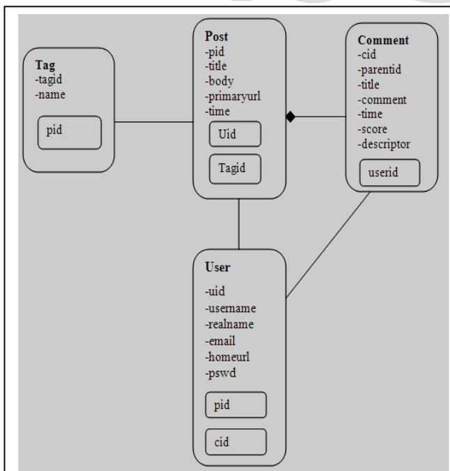
Fig. 1. Class diagram representation of case study
