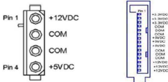
Figure 1. Peripheral power connector and serial ATA connector.
