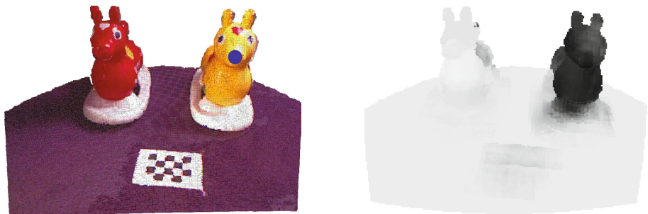
Fig. 9. Color similarity w.r.t. the marked point (blue dot) measured using the saturated Earth Mover’s Distance ( \widehat{\text{EMD}} ) on our color descriptors
