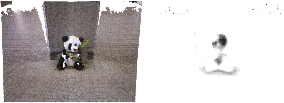
Fig. 10. Luminance similarity w.r.t. the marked point (blue dot) measured using the saturated Earth Mover’s Distance ( \widehat{\text{EMD}} ) on our luminance descriptors
