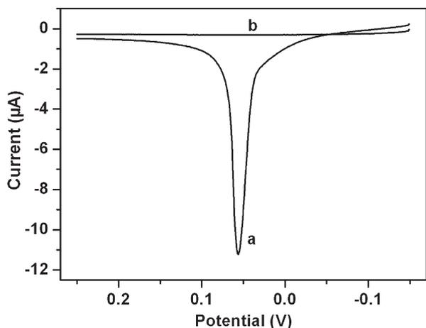
Figure 4. Linear sweep stripping voltammetric curves of Ag NPs deposited at the HIgG immunosensor (a) and neighboring bare electrode (b) in 1.0 M KCl after sandwich-type immunoreactions with 100 ng/mL HIgG and enzymatic silver deposition.
