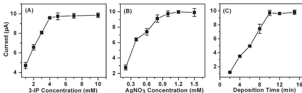
Figure 2. Effects of 3-IP concentration (A),  $\text{AgNO}_3$  concentration (B), and deposition time (C) on stripping current of Ag NPs in 1.0 M KCl.
