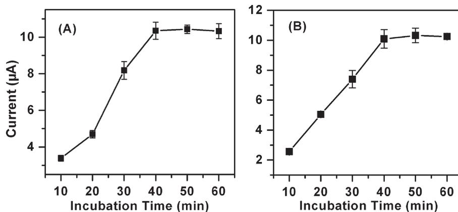
Figure 3. Effect of incubation time on stripping current of Ag NPs in 1.0 M KCl for 100 ng/mL HIgG (A) and MIgG (B).
