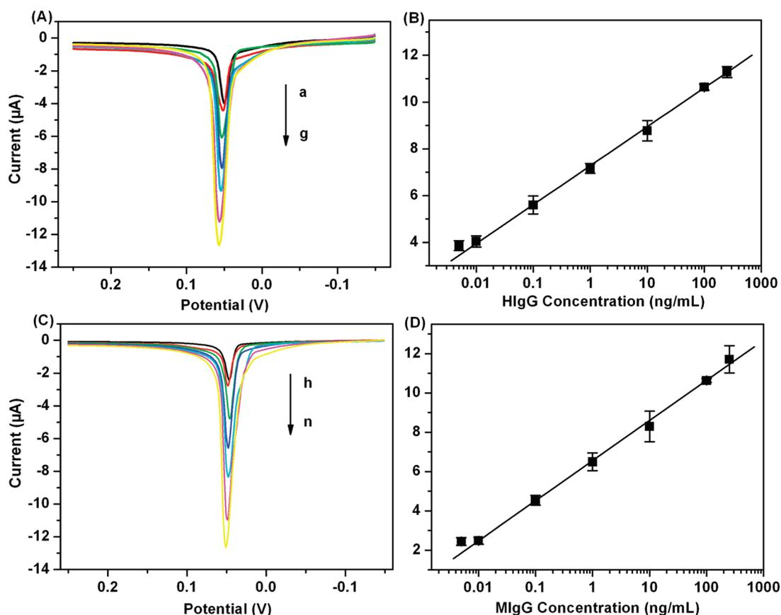
**Figure 6.** Linear sweep stripping voltammetric curves of Ag NPs deposited at immunosensors (A, C) and calibration curves (B, D) for simultaneous multiplexed detection of HlgG (A, B) and MIgG (C, D) using the proposed strategy. Curves a–g and h–n are for 5 pg/mL to 250 ng/mL HlgG and MIgG at W1 and W2, respectively.
