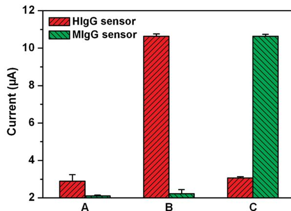
Figure 5. Linear sweep stripping voltammetric responses of the HIgG and MIgG immunosensor array for blank control (A), 100 ng/mL HIgG (B), and 100 ng/mL MIgG (C).
