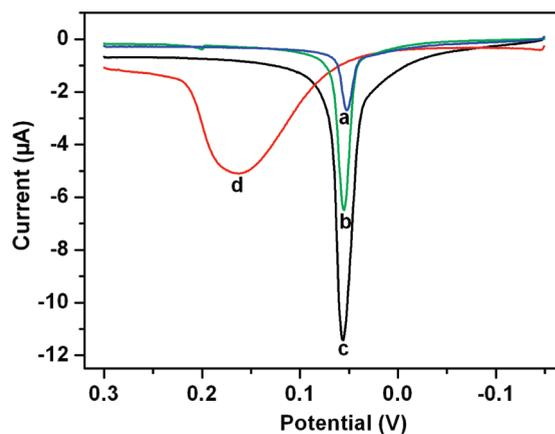
**Figure 1.** Linear sweep stripping voltammetric curves of Ag NPs deposited at HIgG immunosensors after incubation with 0 (a) and 100 ng/mL (b, c, d) HIgG and then ALP-labeled antibody (b) and ALP-labeled antibody/Au NPs (a, c, d) as trace tags at 50 mV s<sup>-1</sup>. The detection solutions were 1.0 M KCl (a, b, c) and 0.1 M HNO<sub>3</sub> containing 0.6 M KNO<sub>3</sub> (d), respectively.
