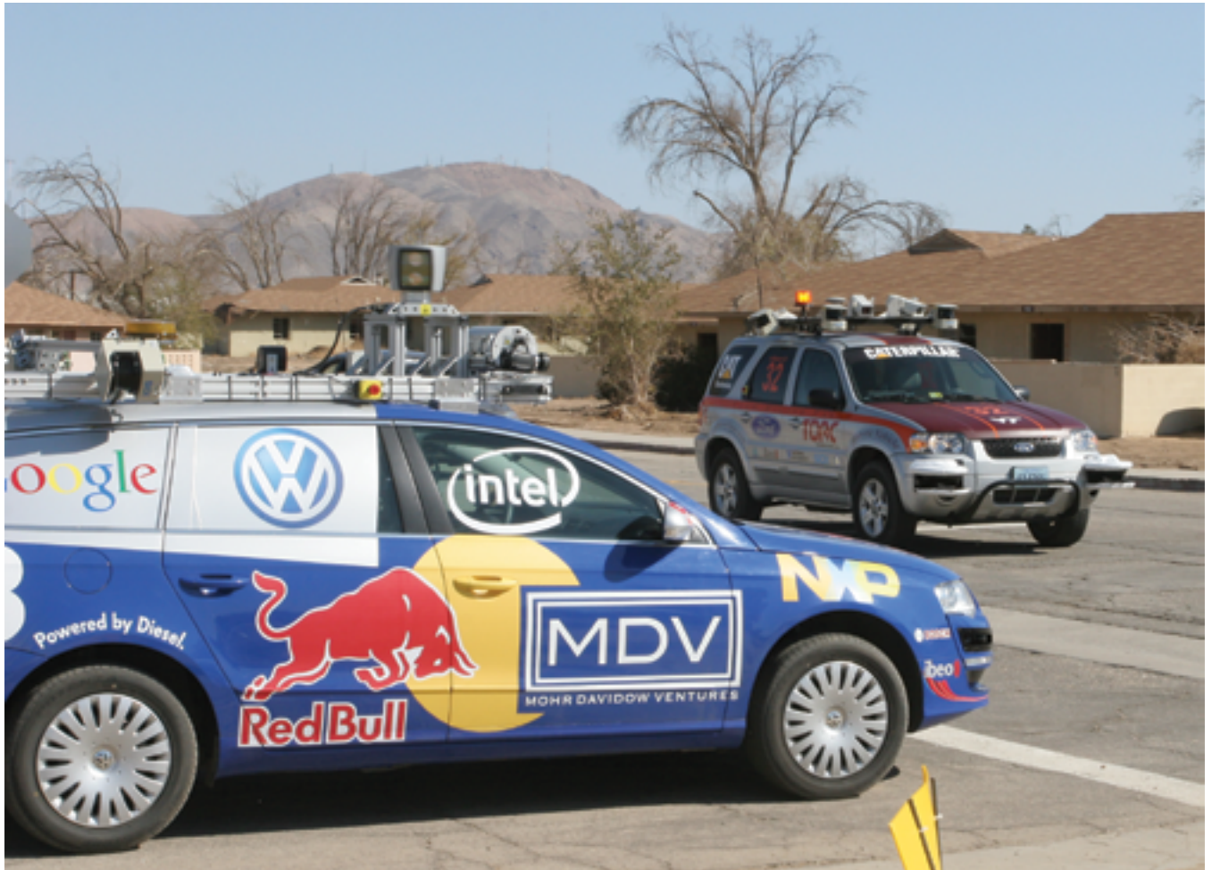
Two driverless automobiles, navigating under computer control, arrive at an intersection in the DARPA Urban Challenge, a contest staged in 2007 by the U.S. Defense Advanced Research Projects Agency. In the foreground is Junior, a vehicle built by a team at Stanford University (and emblazoned with the insignia of its other sponsors). The other vehicle is Odin, from team VictorTango at Virginia Tech, which has the right of way and is proceeding through the intersection. Both vehicles have roof racks bearing multiple cameras, radars and laser scanners, as well as other sensory systems mounted elsewhere. Among 11 finalists, six finished the assigned course. The winner was a team from Carnegie Mellon University; Stanford came in second and Virginia Tech third. The event was held on the streets of George Air Force Base, a decommissioned facility in southern California. (Image courtesy of the Defense Advanced Research Projects Agency.)
