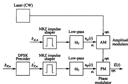
Fig. 2. ASK-DPSK modulator with amplitude and phase path. CW light is first modulated in its amplitude and then in its phase.
