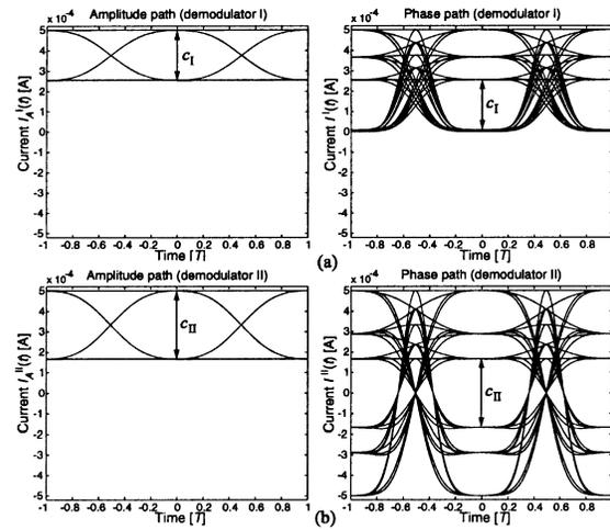
Fig. 4. Eye diagrams after amplitude and phase paths of (a) demodulator I, and (b) demodulator II. ( $P = 1$  mW, ideal photodiodes with  $R = 1$  A/W).
