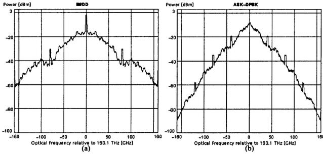
Fig. 5. Spectra of (a) 80-Gb/s IM/DD and (b) 80-Gb/s ASK-DPSK/DD.
