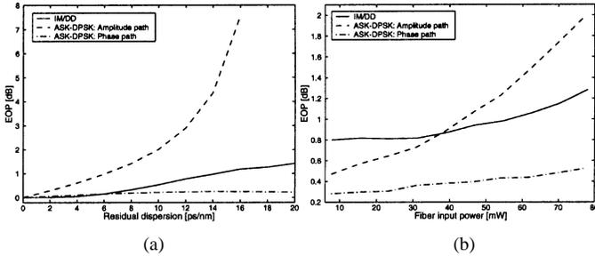
Fig. 6. Comparison of ASK-DPSK/DD and IM/DD. (a) EOP versus residual dispersion for 80-Gb/s IM/DD and 80-Gb/s ASK-DPSK/DD. (b) EOP versus fiber input power for Ch. 5 of an eight-DWDM system with 160-GHz channel spacing for  $8 \times 80$ -Gb/s IM/DD and  $8 \times 80$ -Gb/s ASK-DPSK/DD after 60 km of SMF ( $D = 16$  ps/(nm·km)) at Ch. 5 and 10.67 km of DCF ( $D = -90$  ps/(nm·km)) at Ch. 5).
