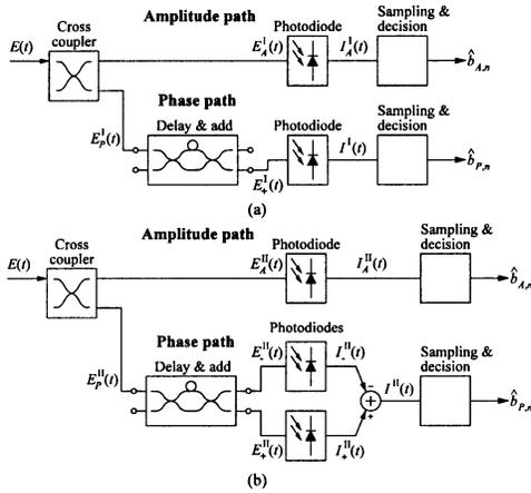
Fig. 3. ASK-DPSK/DD demodulator structures. (a) Demodulator I. (b) Demodulator II.
