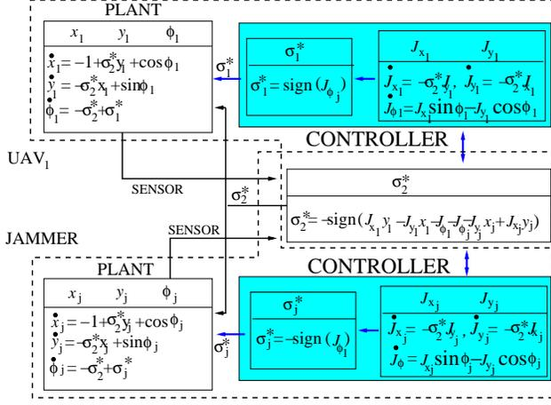
Fig. 3. The Control Loop for the System
