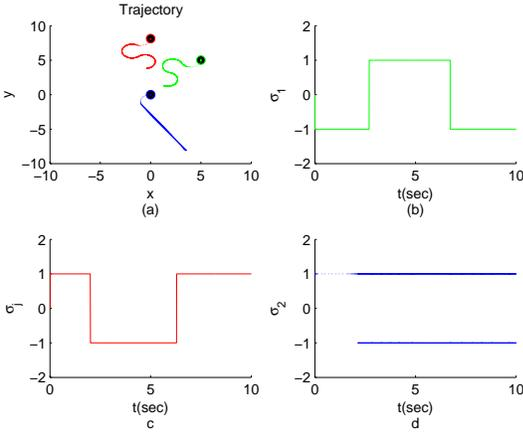
Fig. 5. Figure shows the players leading to Termination condition 2 for Problem 1. The value  $\eta = 2$ . The player in red is the jammer. The players in green and blue are UAV<sub>1</sub> and UAV<sub>2</sub> respectively. Figure (b) shows the control of the UAV<sub>1</sub>. Figure (c) shows the control of the UAV<sub>J</sub>. Figure (d) shows the control of the UAV<sub>2</sub>.
