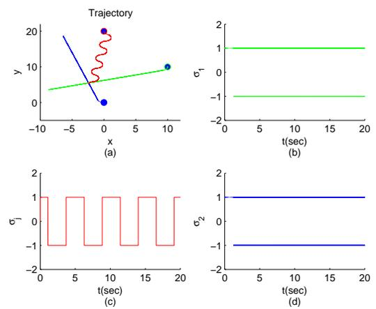
Fig. 7. Figure shows the players leading to Termination condition 2 for Problem 2. The value  $\eta = 1$ . The player in red is the jammer. The players in green and blue are UAV<sub>1</sub> and UAV<sub>2</sub> respectively. Figure (b) shows the control of the UAV<sub>1</sub>. Figure (c) shows the control of the UAV<sub>J</sub>. Figure (d) shows the control of the UAV<sub>2</sub>.
