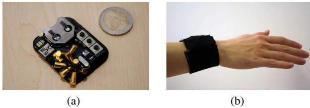
Figure 3. The wearable sensor platform used for recording activities.
