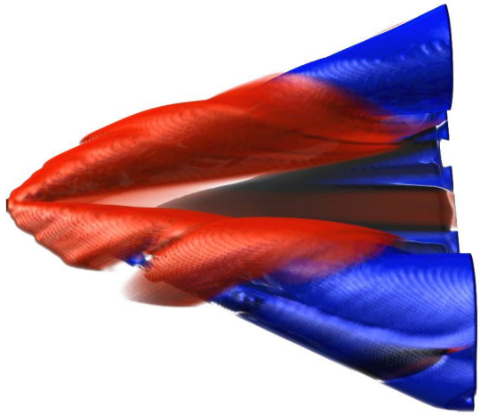
(a) Wing edge separation and the primary attachment layer. Inner structures are occluded.
