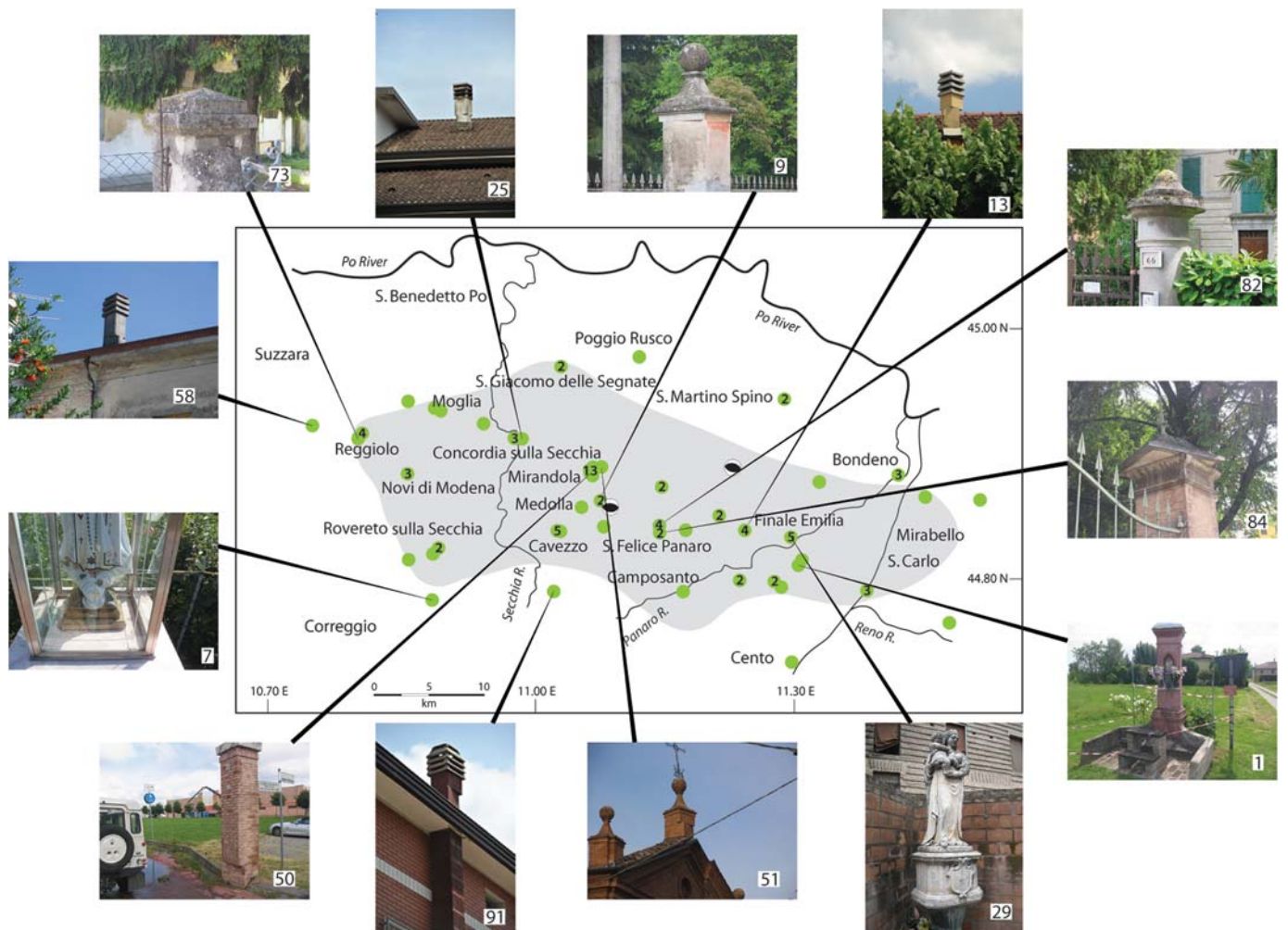
▲ Figure 2. Map of the observation sites of rotational effects and examples of rotations. The numbers inside the green circles indicate multiple observations associated to the same site. The focal mechanisms indicate the epicenters of the 2012 mainshocks. The numbers in the lower right corner of each photo indicate the corresponding record in the \square electronic supplement to this paper. The gray shaded area represents the area of maximum damage ( \text{Int} \geq 6.5 ).
