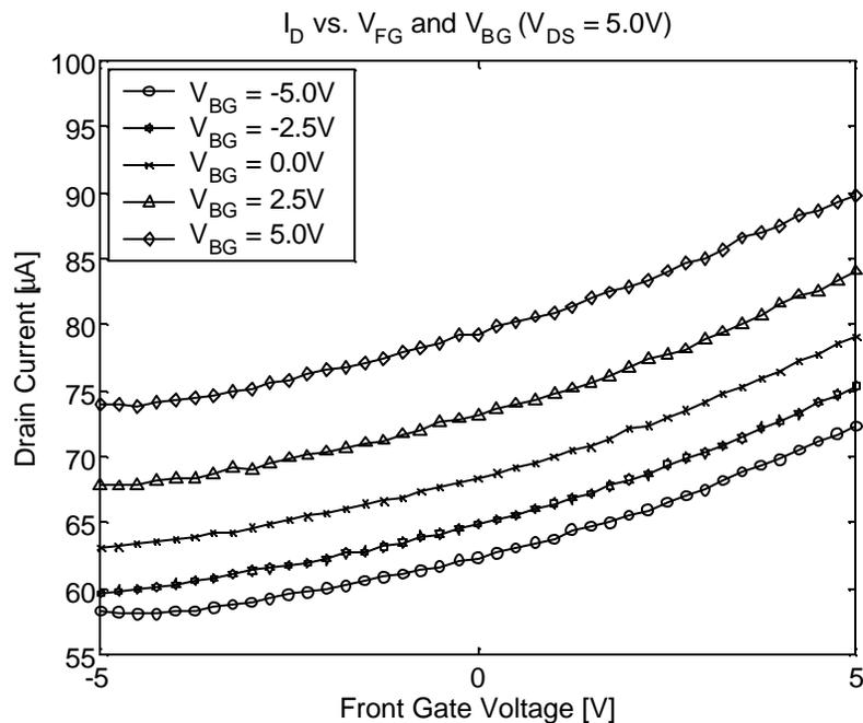
**Figure 65. Example of  $I_D$  vs.  $V_{FG}/V_{BG}$  data from NFET1b process run**
