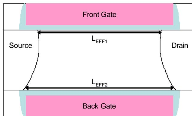
**Figure 21. Effect of Source/Drain implant profile on effective gate lengths of double-gate device**
