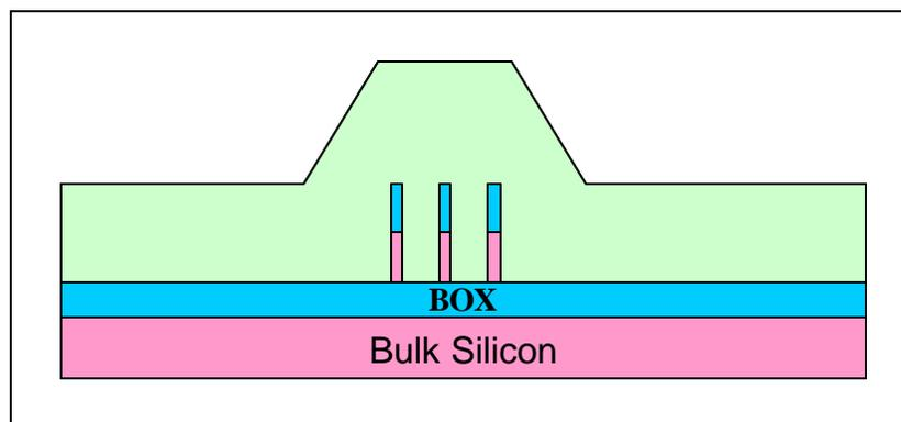
**Figure 49. Illustration of wafer cross section showing relative heights of deposited polysilicon, RX features and outer area of wafer**
