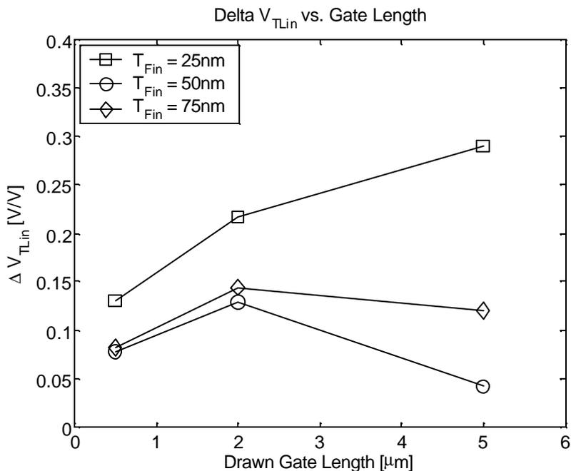
**Figure 83. Change in  $V_{TLIN}$  as a function of device dimensions.**
