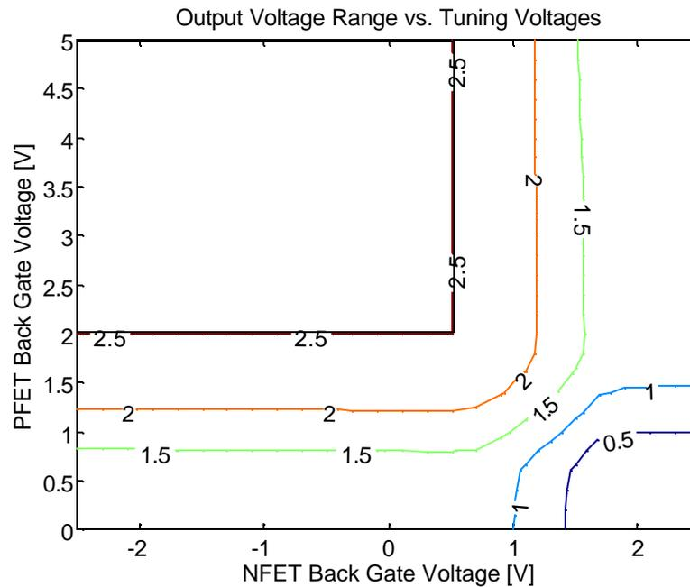
**Figure 25. Output voltage range as a function of back gate voltages for IG-CMOS inverter. The shaded area shows the regime where output voltage swings from rail to rail.**
