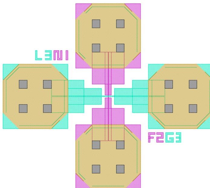
**Figure 36. Testsite layout of single IG-FinFET (Source/Drain are top/bottom, Front/Back Gates are left/right). Octagonal metal pads are designed to optimize packing of devices into an array.**
