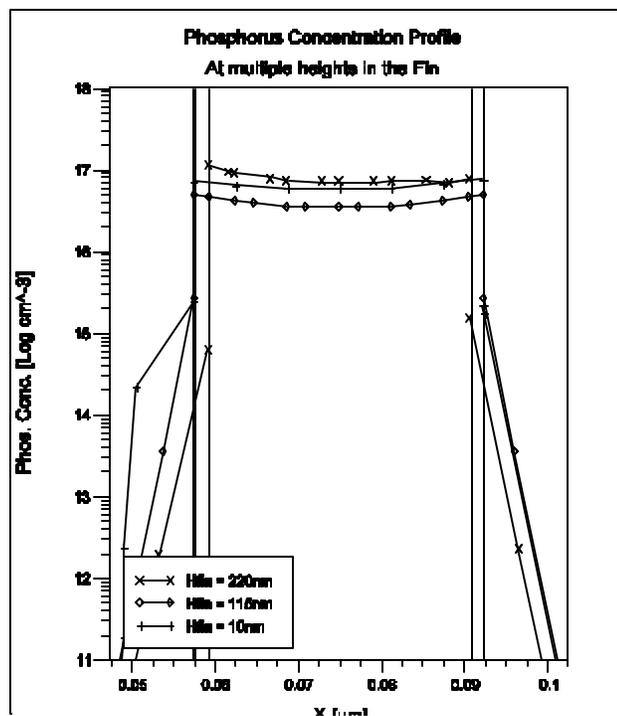
**Figure 44. N-Well Implant profile in 50nm fin after gate thermal oxidation at multiple heights within the fin.**
