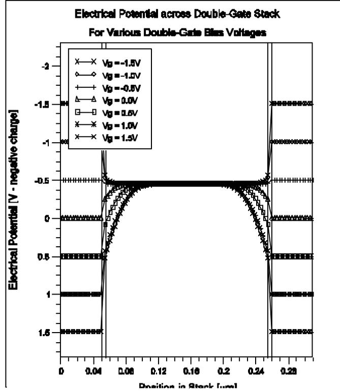
**Figure 8. Simulated potential profile of a thick-body double-gate FET at multiple double-gate bias voltages ranging from accumulation through depletion and into inversion**
