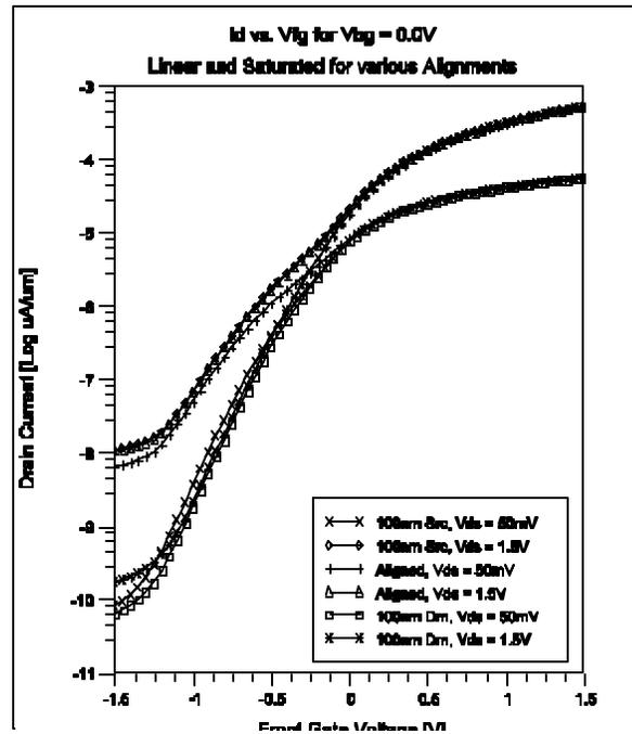
Figure 18. Effect of gate misalignment on independent double-gate device for  $V_{BG} = 0.0V$
