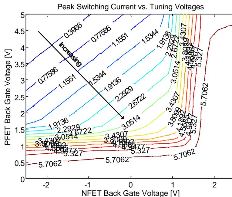
**Figure 26. Peak Switching current as a function of back gate voltages. The arrow indicates the direction of increasing peak switching current in the region of CMOS circuit interest.**
