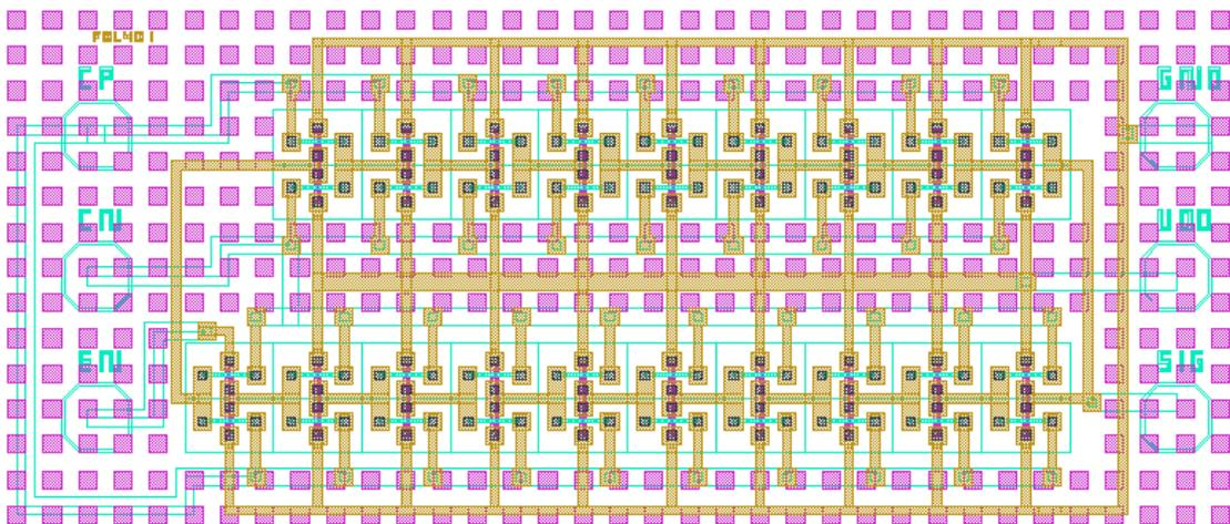
**Figure 39. Testsite layout of IG-FinFET CMOS Tunable Ring Oscillator**
