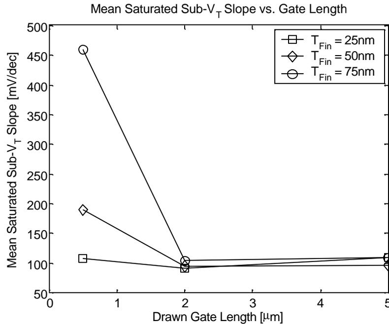
**Figure 74. Mean saturated subthreshold slope vs. drawn gate length for devices fabricated in PFET2c2 process run.**
