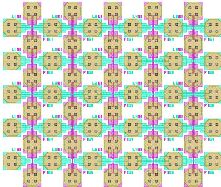
**Figure 37. Testsite array of 25 individually testable single IG-FinFETs**
