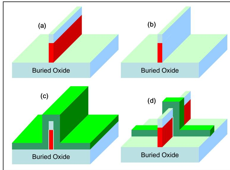
**Figure 6. Fabrication process of a FinFET (a) The fin is etched in SOI. (b) The sidewalls are thermally oxidized. (c) Polysilicon is deposited. (d) The gate electrode is etched.**
