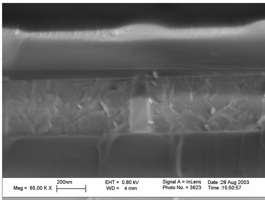
**Figure 53. Cross sectional SEM of Fin with remaining hardmask separating polysilicon gate electrodes**
