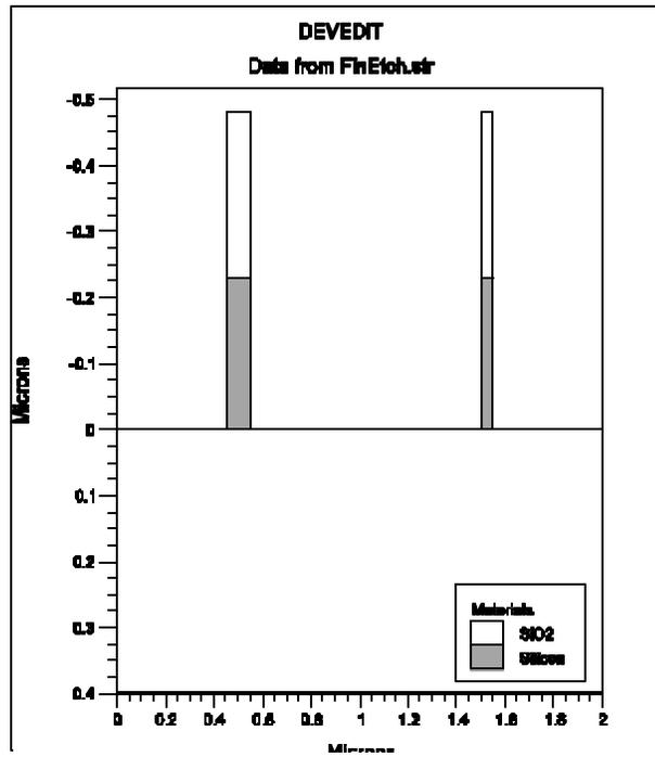
Figure 41. Simulation image of idealized 100nm and 50nm etched silicon fin, with Buried Oxide below and hardmask oxide above.
