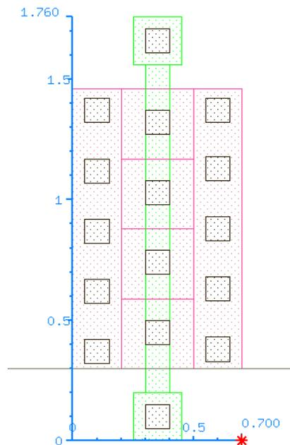
**Figure 32. IG-FinFET single device layout**
