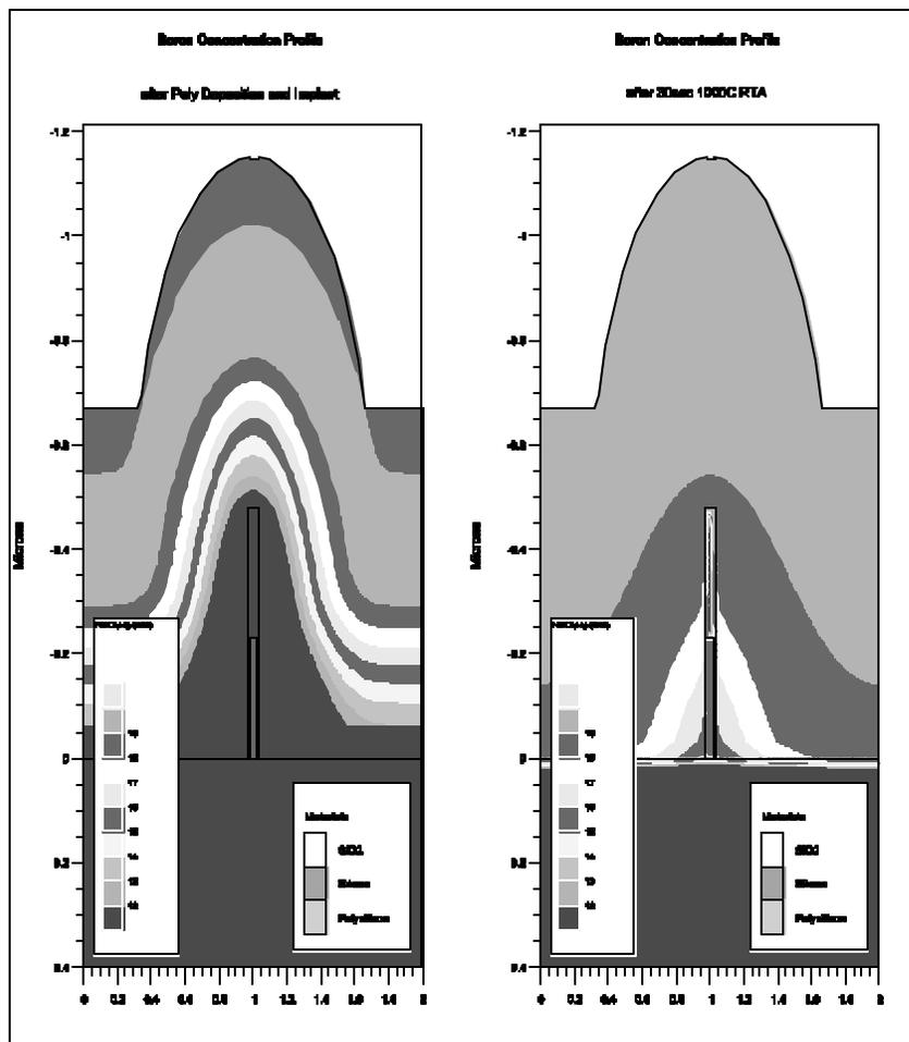
Figure 45. Cross-sectional implant profile simulation results showing Boron concentration in polysilicon gate electrode film after deposition and  $1e15\text{cm}^{-2}$   $80\text{keV}$  Boron<sup>11</sup> implant (left), and after 30 second  $1000^{\circ}\text{C}$  RTA (right).
