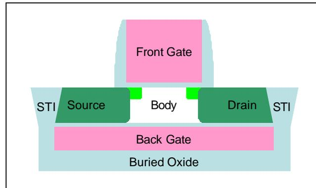
**Figure 17. Cross-sectional structure of the Ground-Plane FET**
