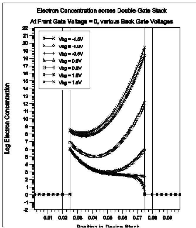
**Figure 13. Simulated electron concentration across a double-gate stack with 50nm thick body with  $1e17 \text{ cm}^{-3}$  Boron doping and symmetric 50Å gate oxides, as the front gate is held at zero potential and the back gate is biased from -1.5V to 1.5V**
