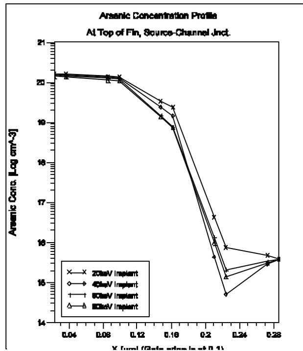
**Figure 63. Arsenic concentration profile in the top of the fin under the gate edge for various implant energies**
