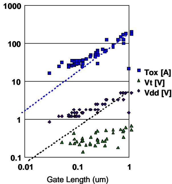
**Figure 2. Industry data showing  $T_{OX}$ ,  $V_T$  and  $V_{DD}$  scaling trends below 1micron gate length [2]**
