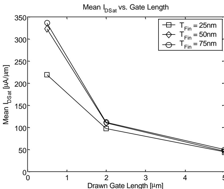
**Figure 78. Mean saturated on-current density ( $I_{DSat}$ ) vs. drawn gate length for devices fabricated in PFET2c2 process run.**
