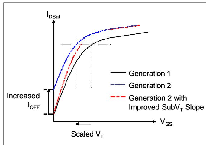
**Figure 1. Idealized  $I_D$  vs.  $V_{GS}$  showing why Subthreshold slope improvement is required when scaling  $V_T$**
