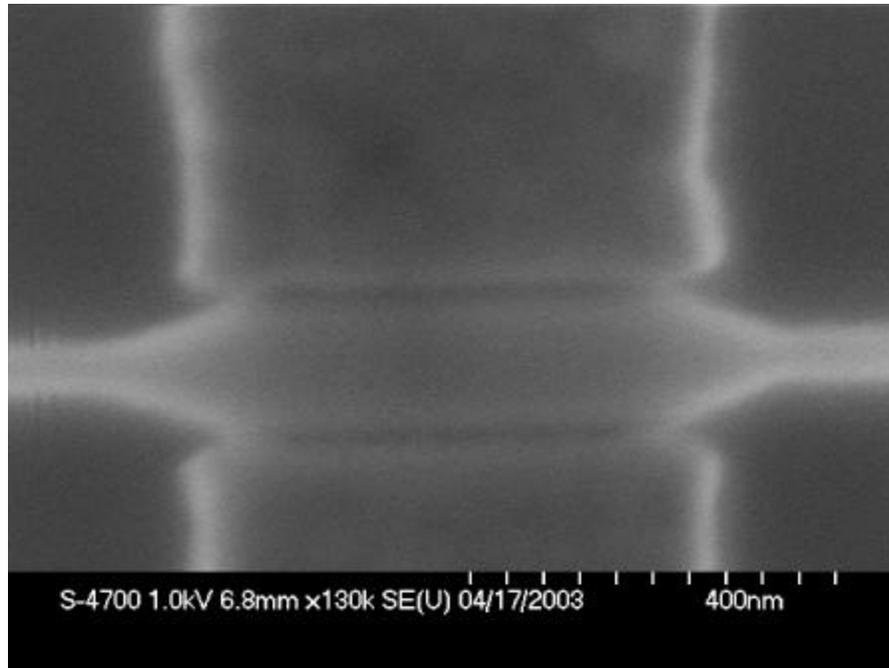
**Figure 55. Top Down SEM of 100nm fin running right to left with 500nm gates on top and bottom from later process run.**
