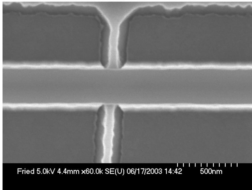
**Figure 56. Top Down SEM showing 75nm fin running from top to bottom and 500nm gates on the left and right from the final process fabrication run**
