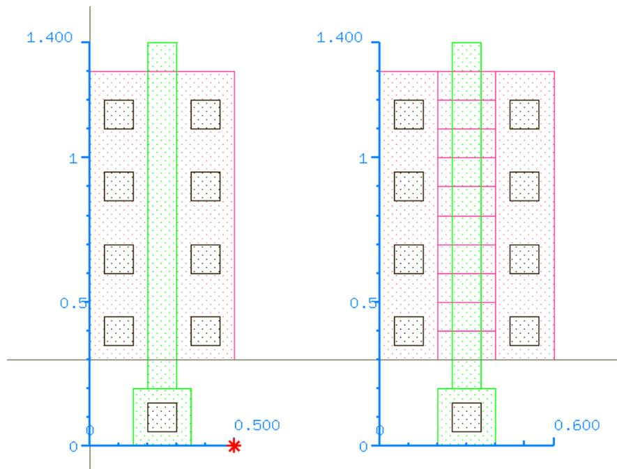
**Figure 31. Planar CMOS layout (a - left) and equivalent FinFET layout (b - right)**
