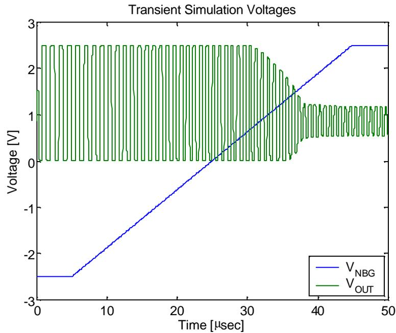
**Figure 29. Results of transient simulation of 19 stage IG-CMOS ring oscillator under varying NFET back gate voltage**
