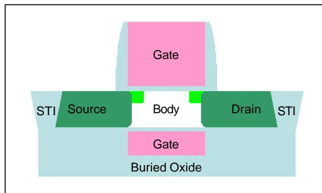
**Figure 5. Structural cross-section of planar double gate FET**
