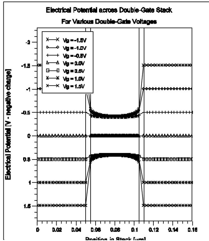
**Figure 11. Potential profile of an undoped-body double-gate FET**
