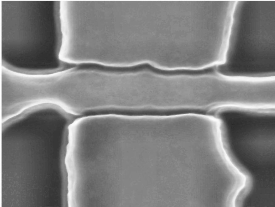
**Figure 54. Top down SEM of 50nm fin running from right to left with 250nm gates on top and bottom from initial fabrication process**
