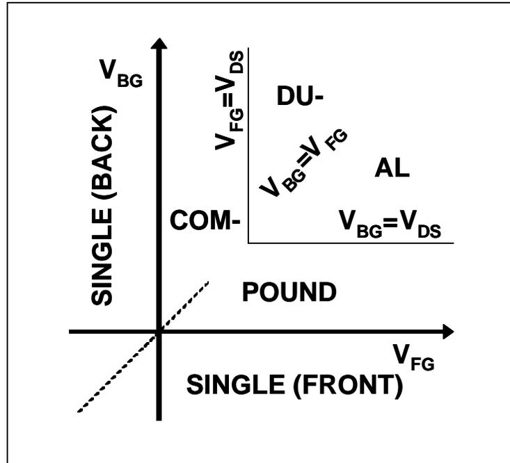
**Figure 22. Partitions of the VFG/VBG plane according to the region of operation of the DGFET [25]**
