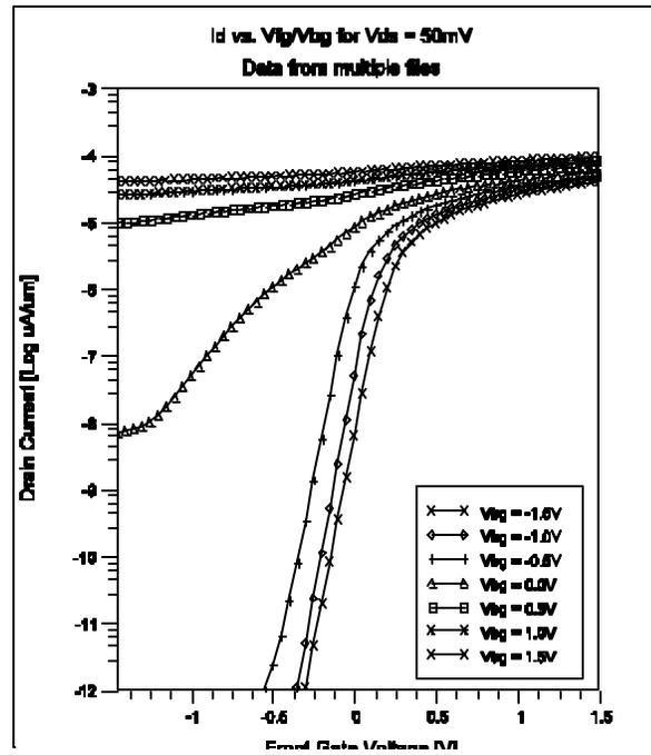
Figure 15. Linear ( $V_{DS} = 50mV$ ) Drain Current as a function of front and back gate bias voltages
