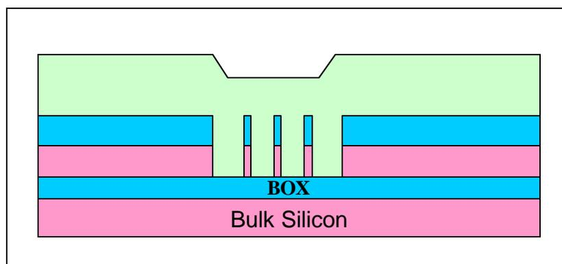
**Figure 50. Illustration of wafer cross section showing relative heights of deposited polysilicon, RX features and outer area of wafer with additional pre-exposure.**
