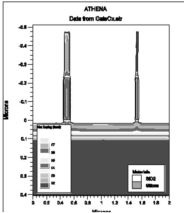
Figure 42. Simulation image showing 100nm and 50nm fin structures after sacrificial oxidation, implant, oxide strip, and gate oxidation.
