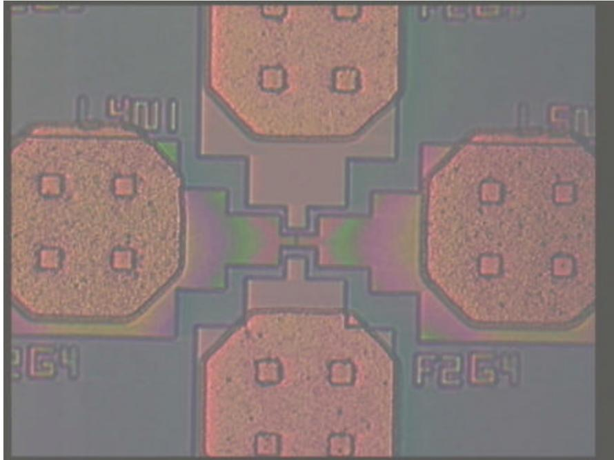
**Figure 64. Top-down micrograph showing etched Aluminum probe pads contacting, via visible contact holes, the gate polysilicon (on right and left) and the single crystal silicon source/drain regions (on top and bottom)**
