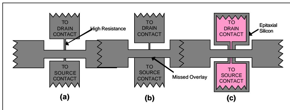
**Figure 35. Effect of extension length variation for overlay tolerance**
