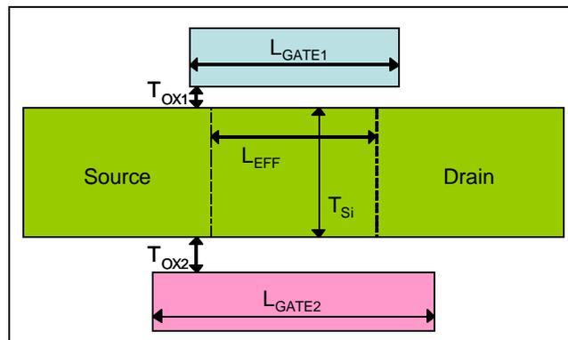
**Figure 7. Structural parameters of interest in a double-gate FET**
