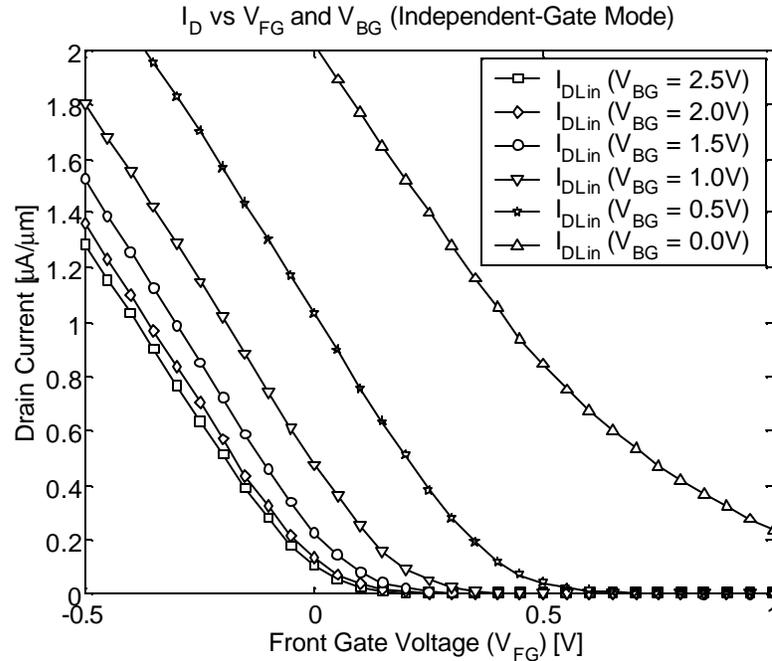
**Figure 81. Linear scale  $I_D$  vs.  $V_{FG}/V_{BG}$  at  $V_{DS} = -50mV$  (linear) for  $T_{FIN} = 50nm$ ,  $L_{GATE} = 0.5\mu m$ ,  $\Gamma = 0.25\mu m$  device from PFET2c2 process run focusing on threshold region.**
