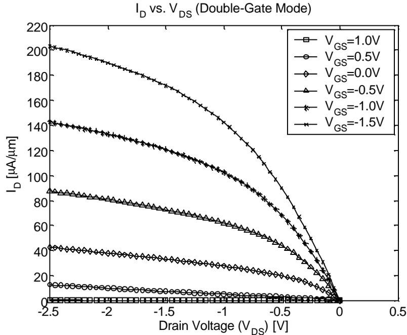
**Figure 72.  $I_D$  vs.  $V_{DS}$  for  $T_{FIN} = 50\text{nm}$ ,  $L_{GATE} = 0.5\mu\text{m}$ ,  $\text{Gamma} = 0.25\mu\text{m}$  device from PFET2c2 process run.**
