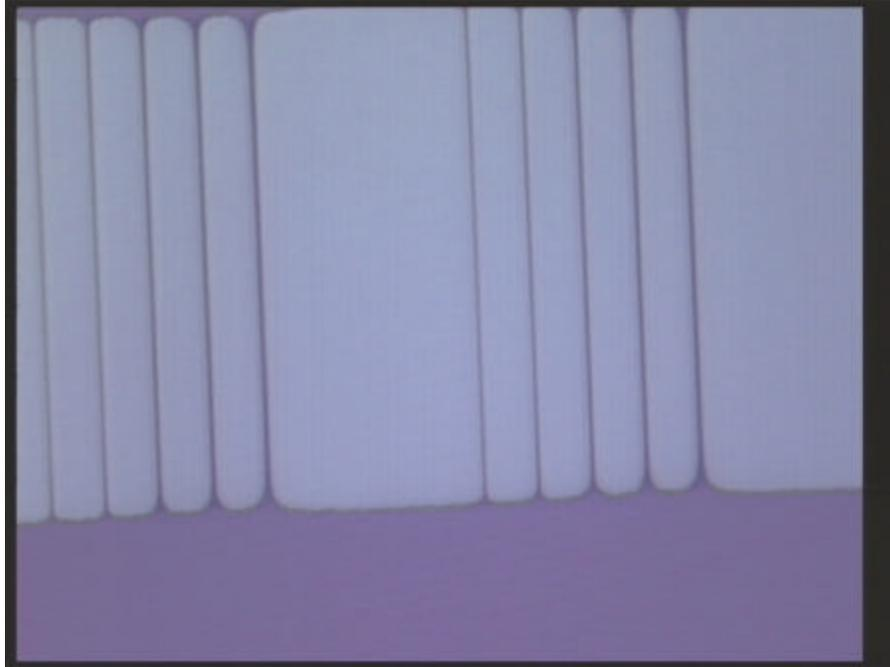
**Figure 40. Top-down micrograph of SEM Macro, showing 10, 25, 50, 75 and 100nm line exposed in NEB-31**
