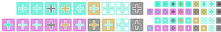
**Figure 87. Structures included on many levels to measure level-to-level overlay**
