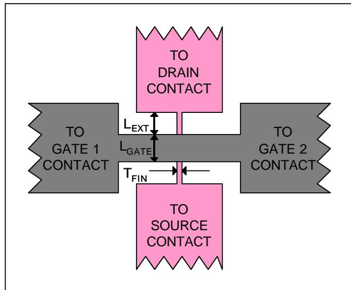
**Figure 34. Three critical dimensions in IG-FinFET individual device layout**
