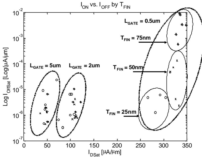
**Figure 79.  $I_{ON}$  vs.  $I_{OFF}$  for all devices sampled in PFET2c2 run**
