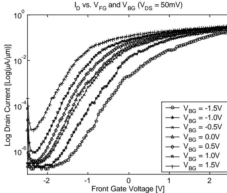
**Figure 67.**  $I_D$  vs.  $V_{FG}/V_{BG}$  at  $V_{DS} = 50\text{mV}$  (linear mode) for  $T_{FIN} = 50\text{nm}$ ,  $L_{GATE} = 2\mu\text{m}$ ,  $\Gamma = 2\mu\text{m}$  device from NFET2a process run. Current is normalized to  $W_{EFF} = 2 \times H_{FIN}$ .
