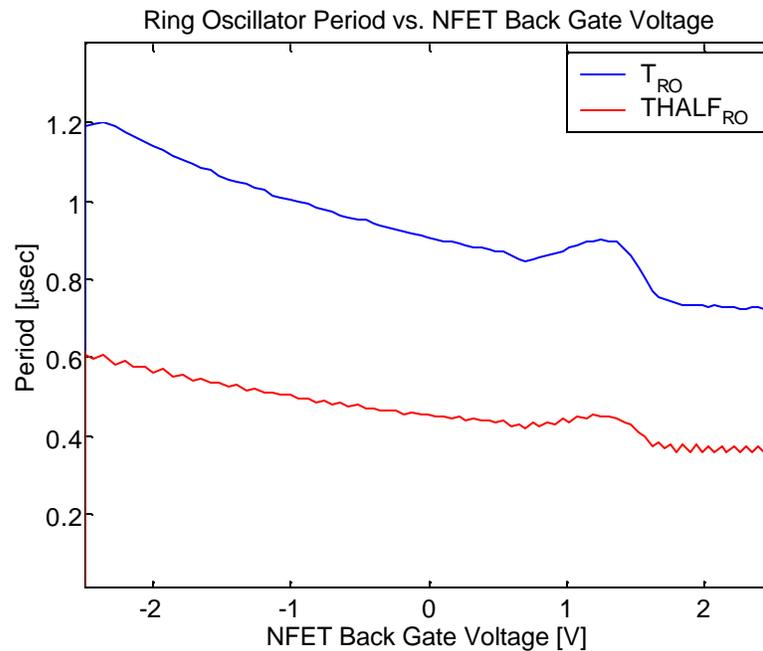
**Figure 30. Extracted simulated ring oscillator period vs.  $V_{NBG}$  for 19 stage IG-CMOS ring oscillator**
