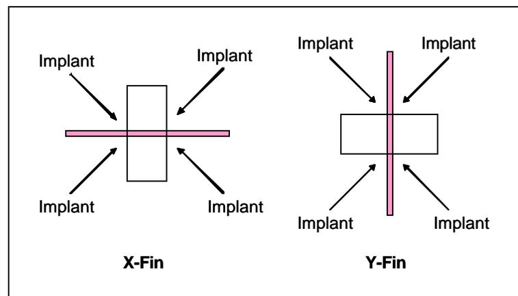
**Figure 57. 45° implant rotations ensure equivalent implants for both X-Fin and Y-Fin oriented FinFETs**
