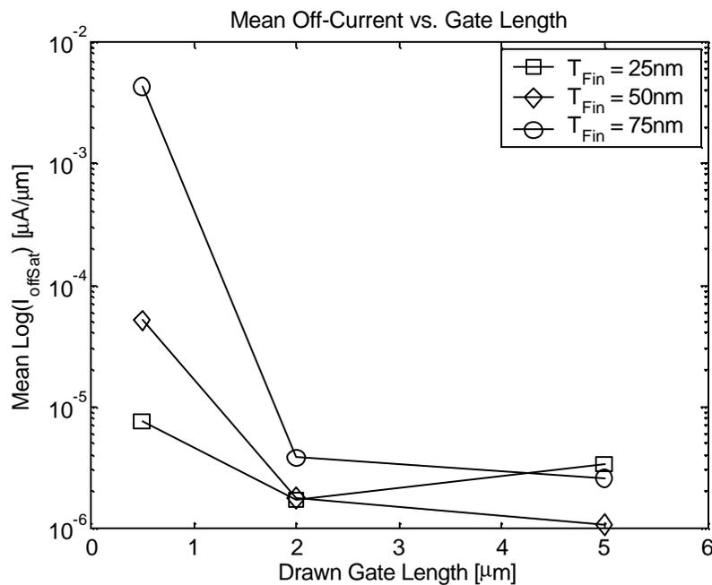
**Figure 77.** Mean saturated off-current density ( $I_{OFFSat}$ ) vs. drawn gate length for devices fabricated in PFET2c2 process run.
