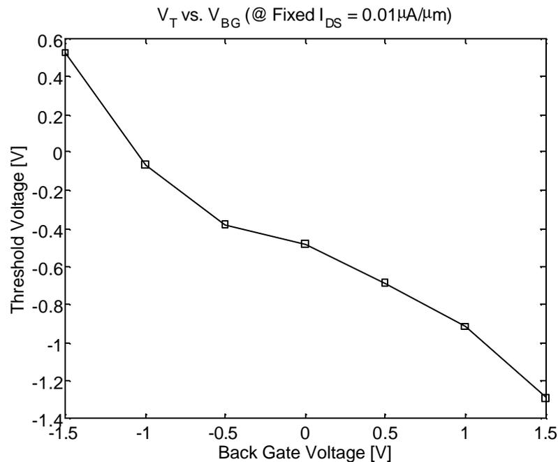
**Figure 68. Extracted threshold voltage vs. back gate voltage**
