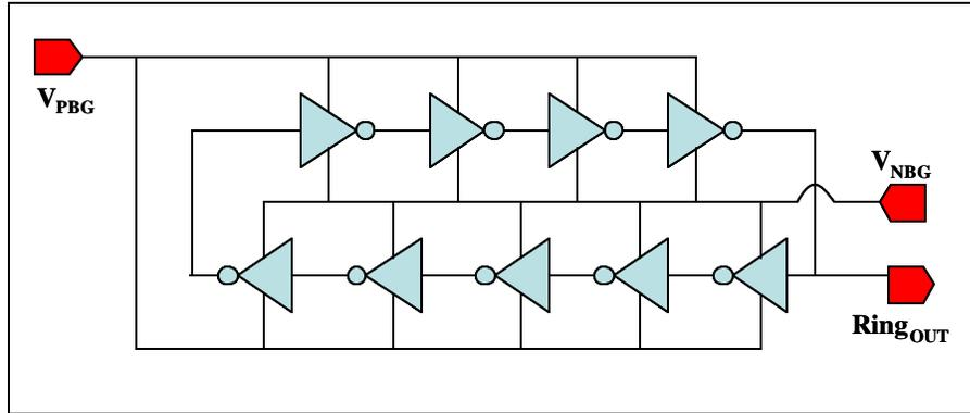
**Figure 28. Schematic representation of a IG-CMOS ring oscillator with all PFET back gates all tied to  $V_{PBG}$  and all NFET back gates tied to  $V_{NBG}$**
