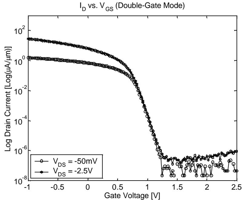
**Figure 71.  $I_D$  vs.  $V_{GS}$   $V_{DS} = -50\text{mV}$  (linear) and  $-2.5\text{V}$  (saturation) for  $T_{\text{FIN}} = 50\text{nm}$ ,  $L_{\text{GATE}} = 2\mu\text{m}$ ,  $\text{Gamma} = 0.25\mu\text{m}$  device from PFET2c2 process run.**
