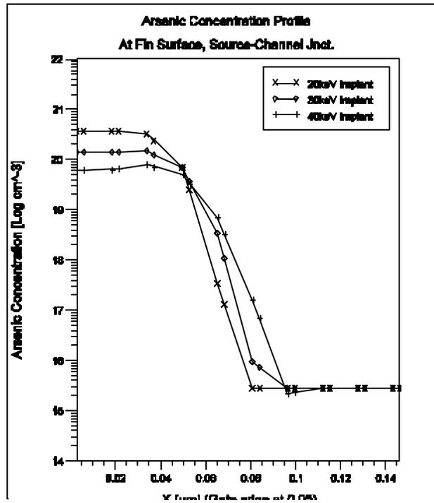
Figure 59. Cut-line analysis of Arsenic concentration profile for multiple energies of implant at the surface of the fin (5nm deep)
