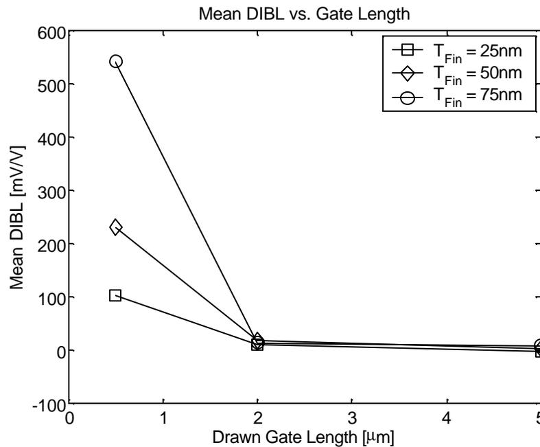
**Figure 75. Mean Drain Induced Barrier Lowering (DIBL) vs. drawn gate length for devices fabricated in PFET2c2 process run.**
