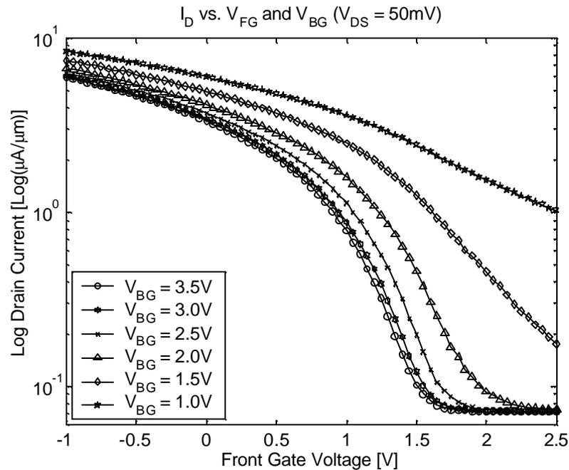
**Figure 69.  $I_D$  vs.  $V_{FG}/V_{BG}$  at  $V_{DS} = -50\text{mV}$  (linear mode) for  $T_{FIN} = 50\text{nm}$ ,  $L_{GATE} = 0.35\mu\text{m}$ ,  $\Gamma = 0.25\mu\text{m}$  device from PFET2c1 process run.**
