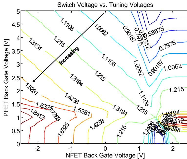
**Figure 27. Inverter transition voltage as a function of back gate voltages. The arrow indicates the direction of increasing switch voltage in the region of CMOS circuit interest.**
