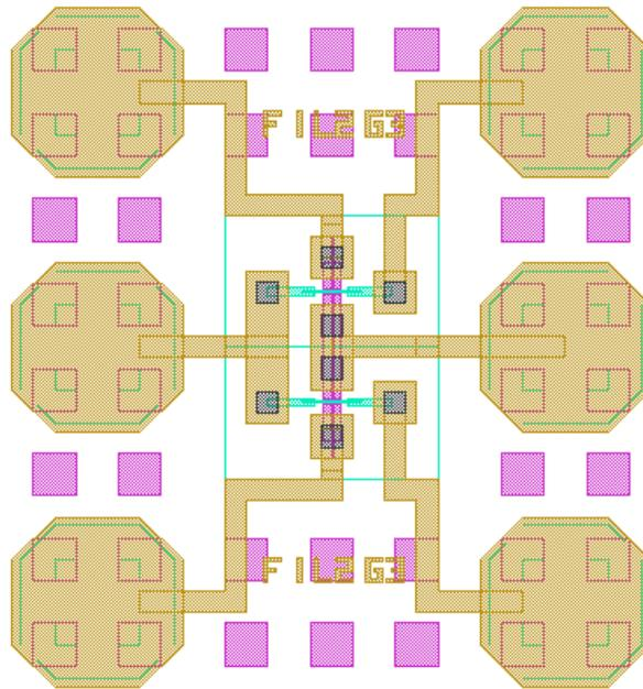
**Figure 38. Testsite layout of IG-FinFET CMOS Inverter**
