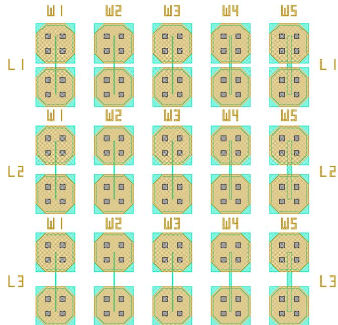
**Figure 89. Polysilicon gate resistance measurement macro design**
