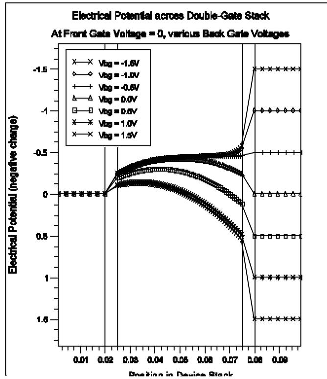
**Figure 12. Simulated electrical potential profile across a double-gate stack with 50nm thick body with  $1e17 \text{ cm}^{-3}$  Boron doping and symmetric 50Å gate oxides, as the front gate is held at zero potential and the back gate is biased from -1.5V to 1.5V**
