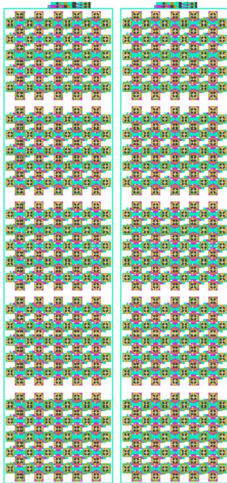
**Figure 85. Device Arrays (NFETs on left, PFETs on right)**
