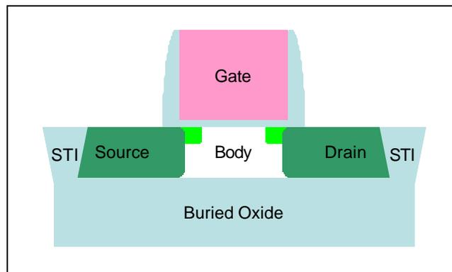
**Figure 3. Structural cross-section of Silicon on Insulator (SOI) Device**
