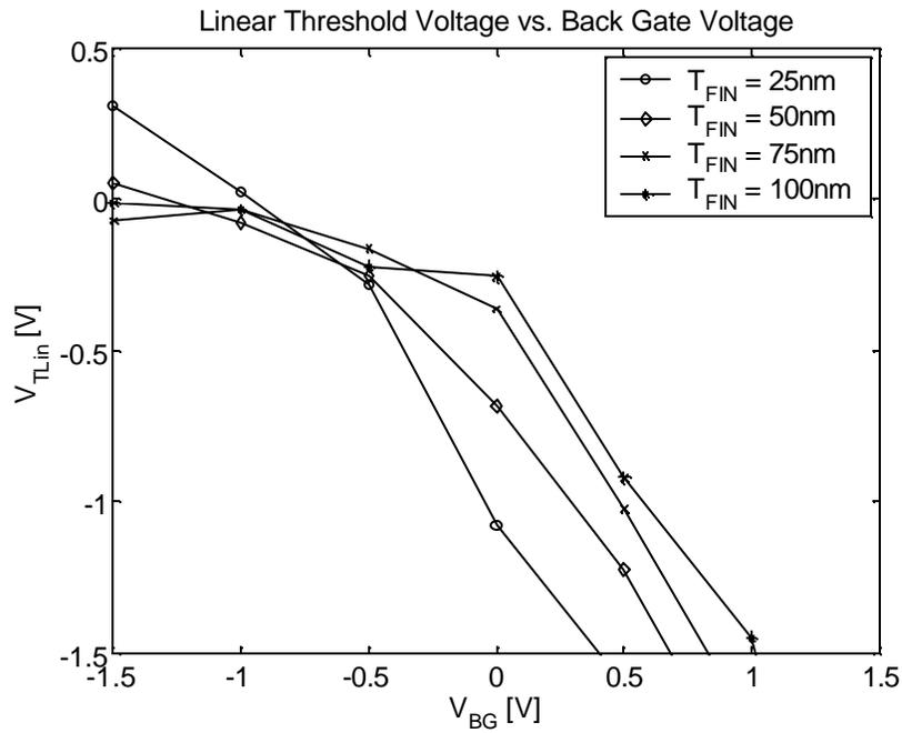
**Figure 19. Simulated Linear Threshold Voltage vs. Back Gate Voltage for n-type IG-FinFETs of various fin thickness**
