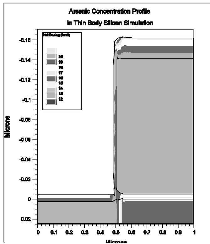
**Figure 58. Cross-sectional Arsenic concentration profile from simulation results using thin body (25nm body thickness before sidewall reoxidation) planar FET and angle-adjusted 40keV implants after sidewall reoxidation and implant**
