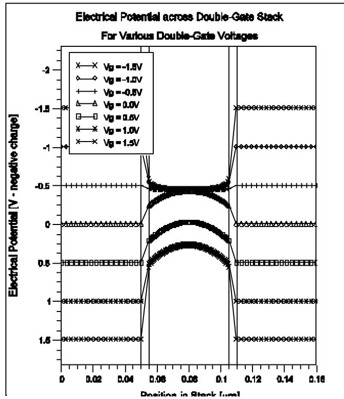
**Figure 9. Simulated potential profile of a thin-body (fully-depleted) double-gate FET at multiple double-gate bias voltages ranging from accumulation through depletion and into inversion**
