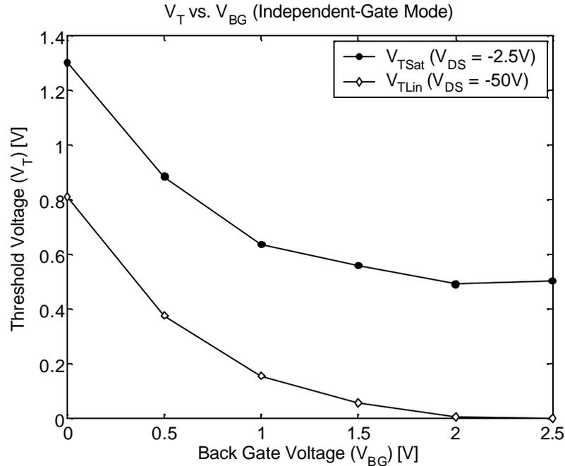
**Figure 82. Threshold Voltage vs. Back-Gate Voltage for  $T_{FIN} = 50nm$ ,  $L_{GATE} = 0.5\mu m$ ,  $\Gamma = 0.25\mu m$  device from PFET2c2 process run.**
