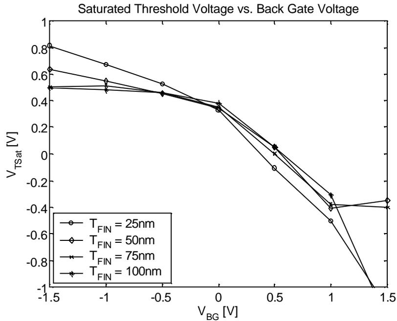
**Figure 20. Simulated Saturated Threshold Voltage vs. Back Gate Voltage for n-type IG-FinFETs of various fin thickness**
