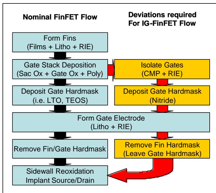
**Figure 33. Process flow for nominal FinFET fabrication and deviations required for Independent-Gate FinFET fabrication**
