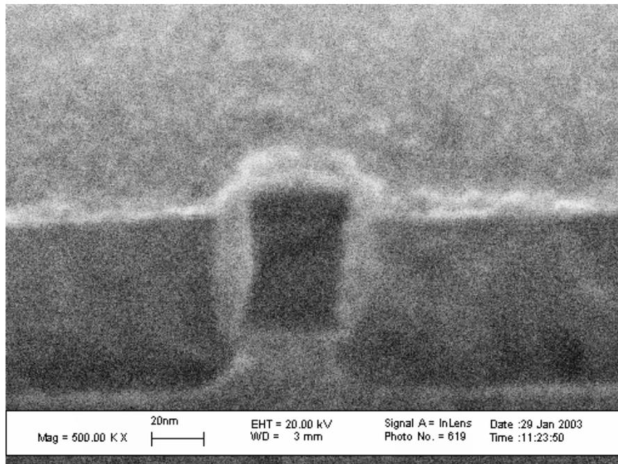
**Figure 48. Cross-sectional SEM image showing the fin, remaining hardmask oxide and two independent gate electrodes.**
