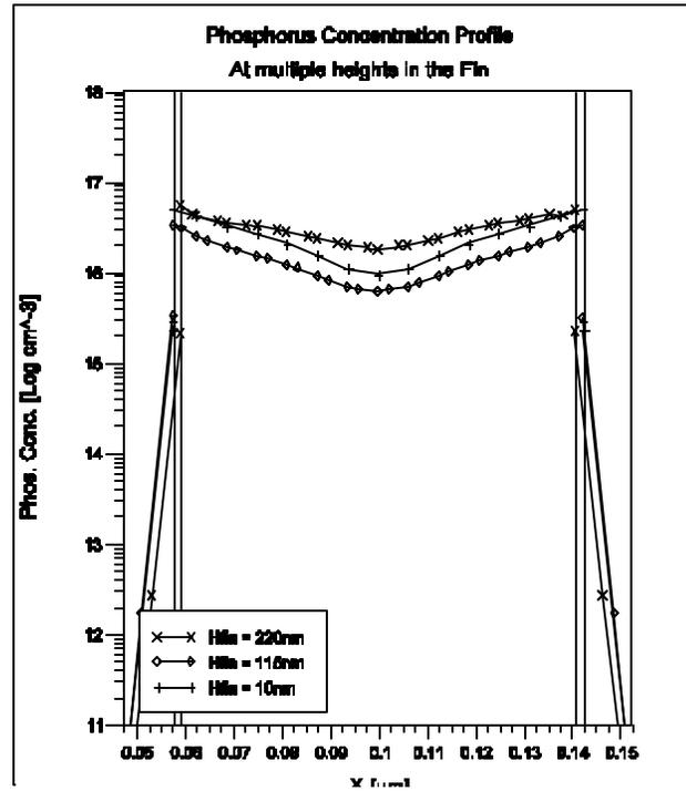
**Figure 43. N-Well Implant profile in 100nm fin after gate thermal oxidation at multiple heights within the fin.**
