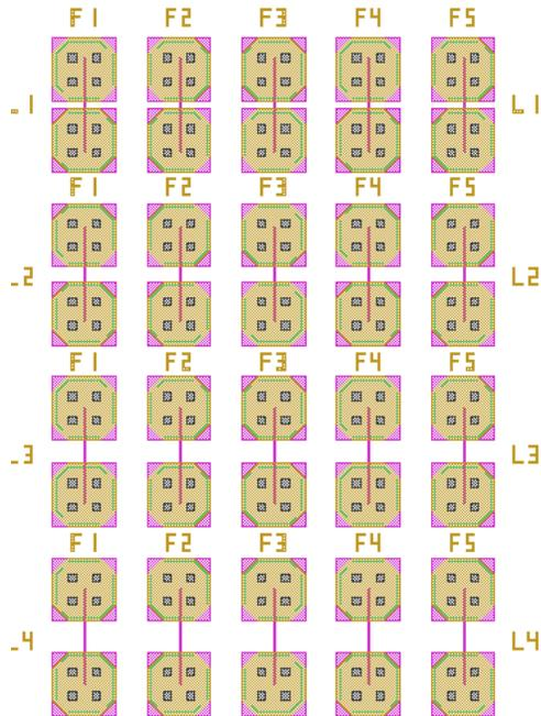
**Figure 88. Fin resistance measurement macro design**
