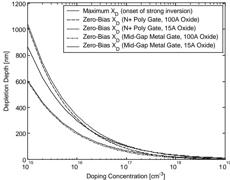
**Figure 10. Depletion depth vs. doping level for different gate stacks**
