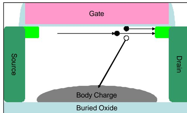
**Figure 4. Cross section of active device area showing impact ionization and the body effect**
