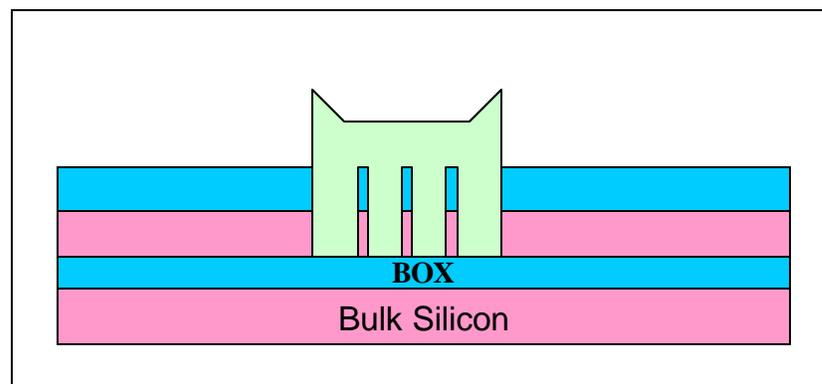
**Figure 51. Illustration of wafer cross section showing relative heights of deposited polysilicon, RX features and outer area of wafer with additional pre-exposure and post-deposition non-critical polysilicon removal.**
