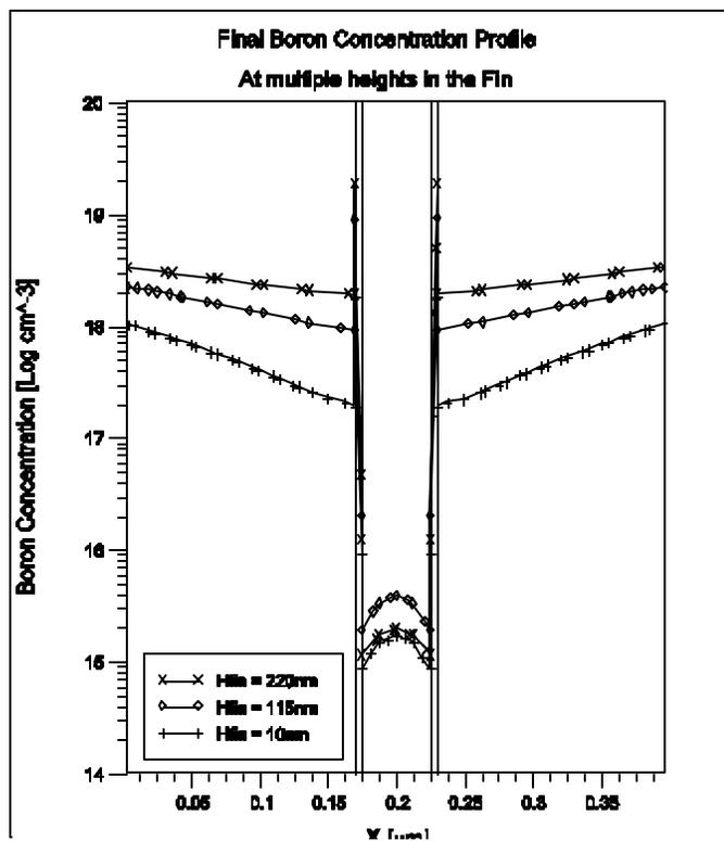
**Figure 47. Cross-sectional cut-line analysis of final Boron concentration in gate electrode at multiple heights in the fin**
