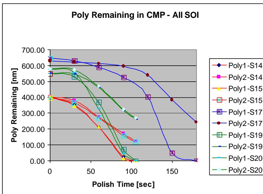
**Figure 52. Data from CMP experiment showing thickness of polysilicon on "high" and "low" features used to determine selectivity and process time.**
