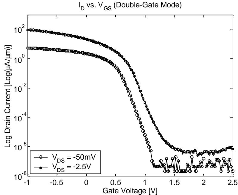
**Figure 70.  $I_D$  vs.  $V_{GS}$  at  $V_{DS} = -50\text{mV}$  (linear) and  $-2.5\text{V}$  (saturation) for  $T_{FIN} = 50\text{nm}$ ,  $L_{GATE} = 0.5\mu\text{m}$ ,  $\text{Gamma} = 0.25\mu\text{m}$  device from PFET2c2 process run.**
