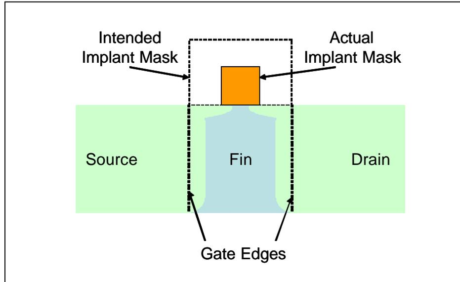
**Figure 66. Side view of hypothesized structure of reduced implant mask, and resulting source/drain implant profiles**
