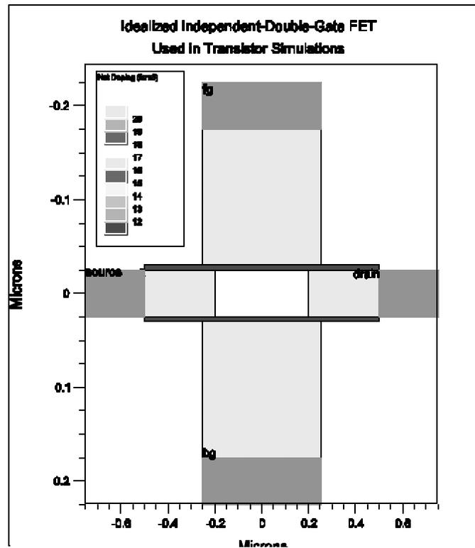
**Figure 14. Idealized Independent Gate Device Structure used in transistor simulations with  $T_{FIN} = 50\text{nm}$  and  $L_{GATE} = 500\text{nm}$  with 50nm symmetric S/D Overlap,  $1e17$  Boron body doping, and  $1e20$  Arsenic doping in the Source/Drain and both gates**
