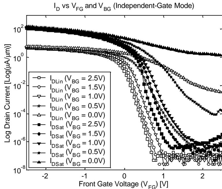
**Figure 80.**  $I_D$  vs.  $V_{FG}/V_{BG}$  at  $V_{DS} = -50\text{mV}$  (linear) and  $-2.5\text{V}$  (saturation) for  $T_{FIN} = 50\text{nm}$ ,  $L_{GATE} = 0.5\mu\text{m}$ ,  $\Gamma = 0.25\mu\text{m}$  device from PFET2c2 process run.
