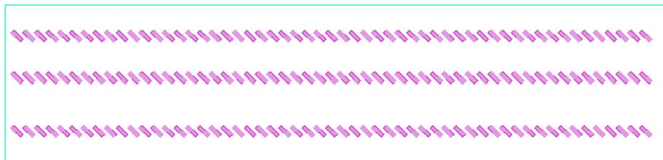
**Figure 86. Structures included on RX level to permit DUV alignment to e-beam written features**
