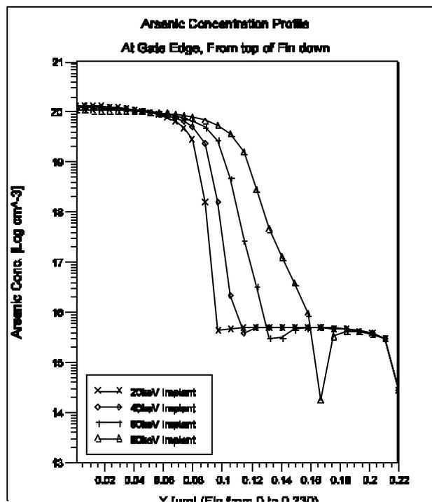
**Figure 62. Top-Down Arsenic concentration profile at the gate edge showing depth of implant as a function of implant energy**
