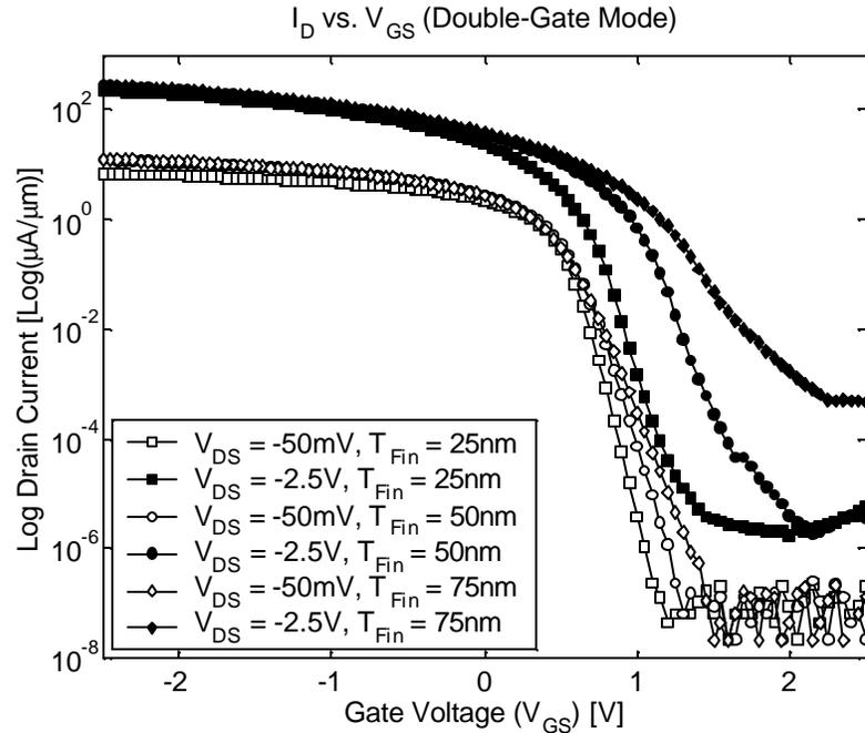
**Figure 73.  $I_D$  vs.  $V_{GS}$   $V_{DS} = -50\text{mV}$  (linear) and  $-2.5\text{V}$  (saturation) for multiple  $T_{FIN}$  dimensions,  $L_{GATE} = 0.5\mu\text{m}$ ,  $\Gamma = 0.25\mu\text{m}$  device from single die on PFET2c2 process run.**
