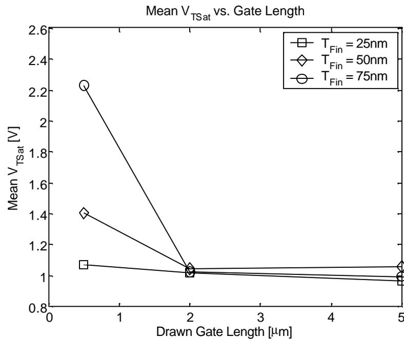
**Figure 76.** Mean saturated threshold voltage ( $V_{TSat}$ ) vs. drawn gate length for devices fabricated in PFET2c2 process run.
