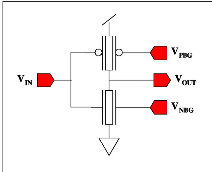
**Figure 24. Circuit schematic of Independent gate CMOS inverter**
