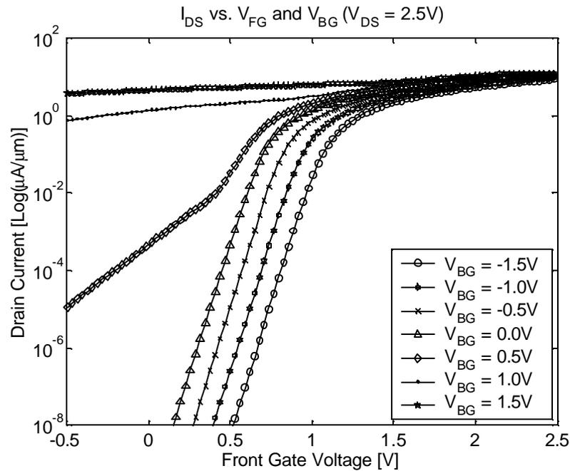
**Figure 23. Simulated  $I_D$  vs.  $V_{FG}/V_{BG}$  curves for an NFET of  $T_{FIN} = 100\text{nm}$ ,  $L_{GATE} = 2\mu\text{m}$ , and symmetric source and drain extension lengths of  $2\mu\text{m}$ , using the converted, adjusted compact DGFET model.**
