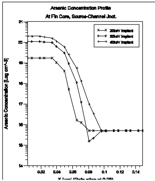
Figure 60. Cut-line analysis of Arsenic concentration profile for multiple energies of implant at the core of the fin (24nm deep)
