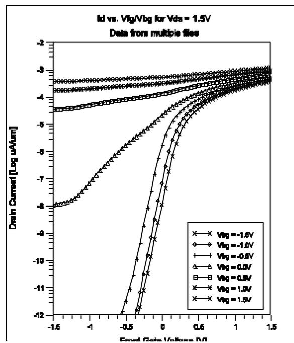
Figure 16. Saturation ( $V_{DS} = 1.5V$ ) Drain Current as a function of front and back gate bias voltages
