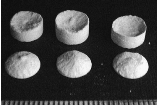
Fig. 3. A photography of broken flat-faced cylindrical tablets [1] showing the cone capping failure pattern.
