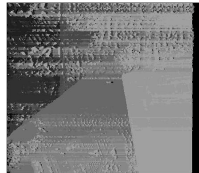
c) Output of traditional local area based correspondence algorithm for color images
