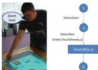
FIGURE 1. Left: End-user interacting with a multimodal system. Right: Visual model used for specifying human-machine interaction.
