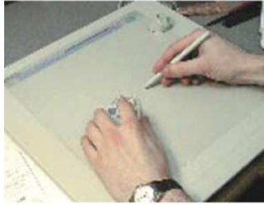
FIGURE 14. Left: Two-handed interaction technique on a tablet. Right: Solid and dashed arcs represent the events generated by the pencil and puck, respectively. The black token can only be in solid states ( b_0 , b_1 , b_2 or bg_3 ) and the gray one, in dashed states ( g_0 , g_1 , g_2 or bg_3 ). States g_0 , g_1 and g_2 indicate the puck's possible situations: off the tablet, in contact with the tablet or being clicked, respectively. States b_0 , b_1 and b_2 have an analogous interpretation for the pen. [Images from (Hinckley et al. , 1998), reproduced with permission.]
