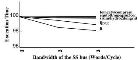
Figure 7: Effect of the SS bus bandwidth.
