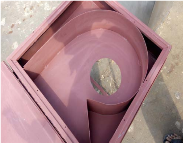
Figure 4: Inner circular duct
