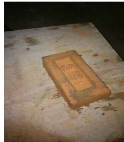
Figure 4: CSEB with Sand (70%) + Clay (20%) + Lime (10%)
