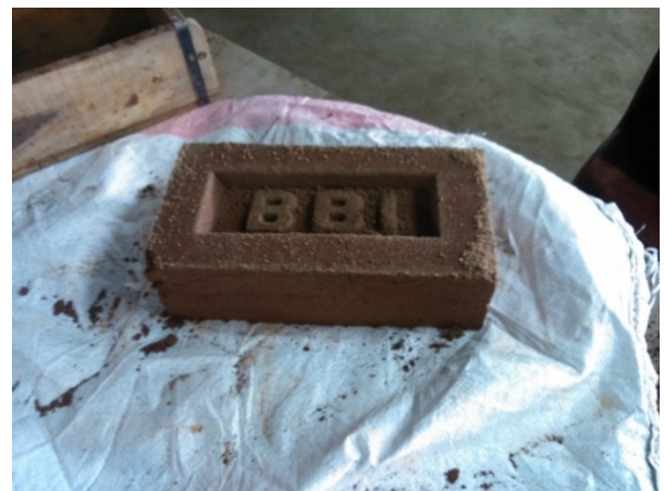
Figure 5: CSEB with Sand (70%) + Clay (30 %)
