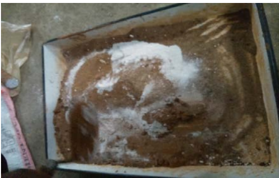
Figure 2: Mix of lime, sand & clay
