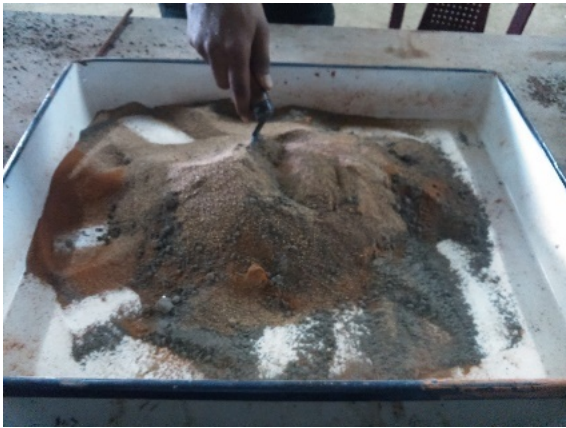
Figure 1: Mix of sand, clay & OPC
