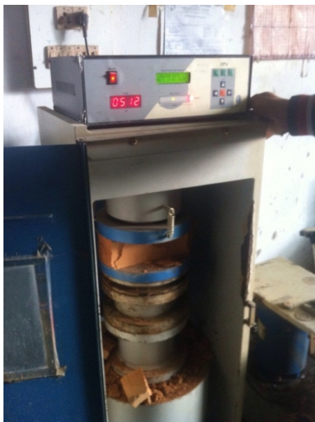
Figure 6: Breaking of CSEBs in CTM
