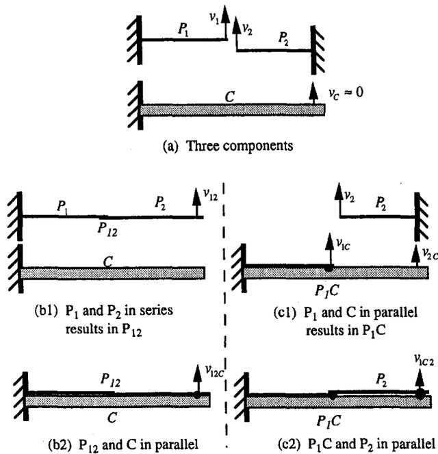
Fig. 6 Two assembly sequences
