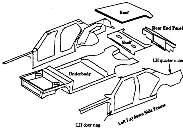
Fig. 1 Automotive body panel structure
