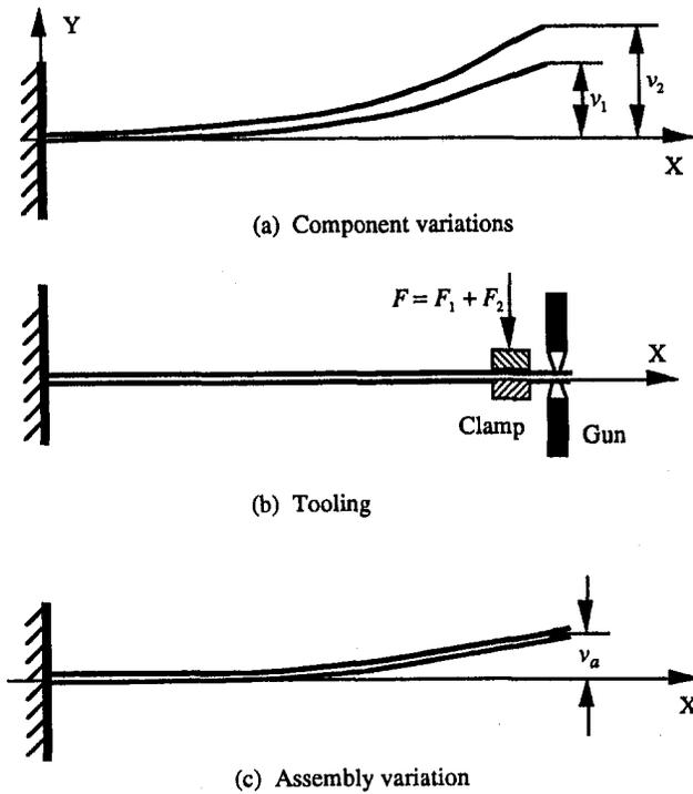
Fig. 4 Assembly in parallel
