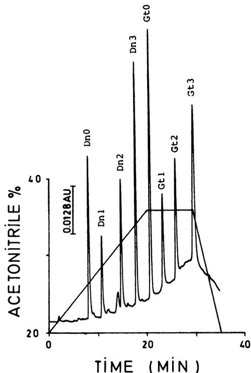
FIG. 2. HPLC separation of gitoxin derivatives.
