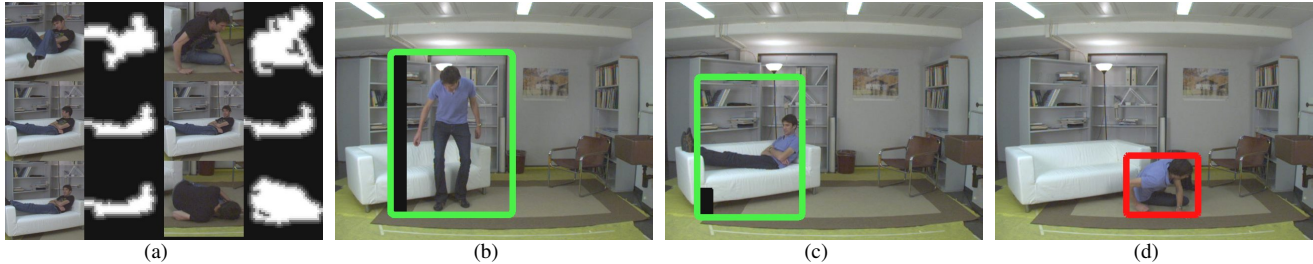
Figure 8. Illustration of the update procedure: (a) some feature vectors and their according image regions taken for the update of H1 , (b) normal appearances stay normal after the update, (c) lying turned normal after the update and (d) real outliers are still detected.
