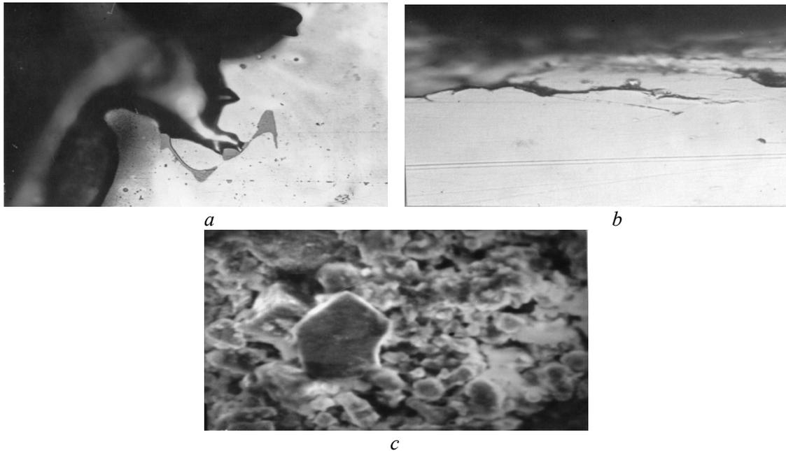
**Figure 3.** Formation of wear particles in areas of sulfide red shortness on the tread surface of railway wheels, x 600
