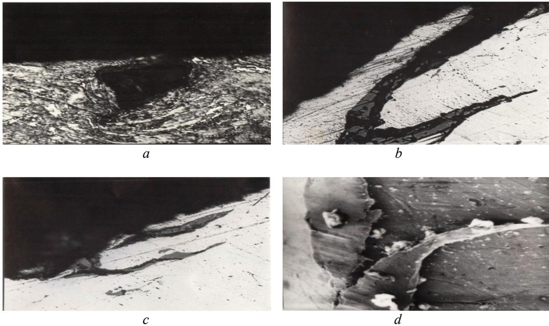
**Figure 2.** Deformation localization (*a*) and formation of wear particles near nonmetallic inclusions and products of wheel steel corrosion (*b-d*) on a tread surface of railway wheels: *a, b* –  $\times 400$ ; *c, d* –  $\times 200$
