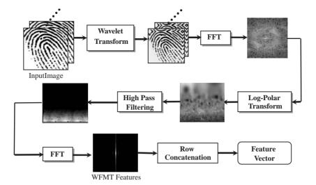
Fig. 2. Block diagram of generating the WFMT features,  $\Gamma$ .
