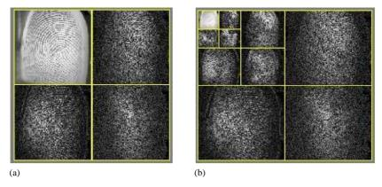
Fig. 1. 2D wavelet decomposition of a fingerprint image: (a) 1-level wavelet decomposition and (b) 3-level wavelet decomposition.
