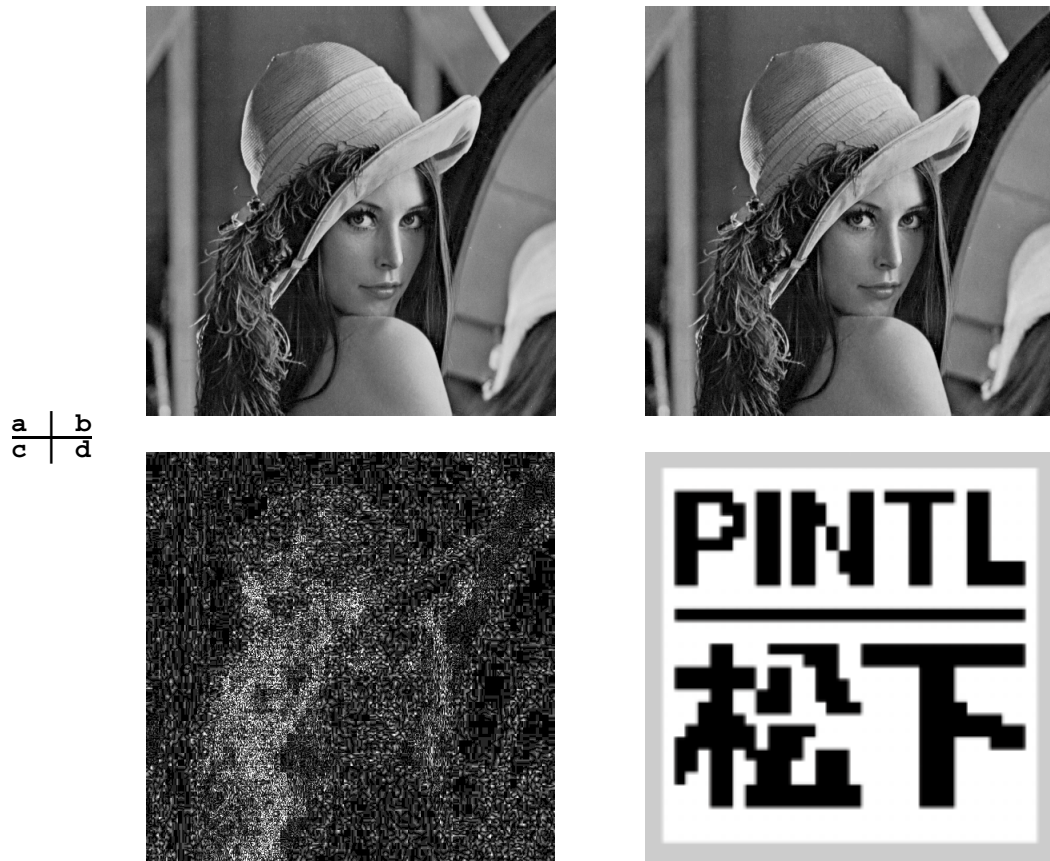
Figure 6.9: \frac{a|b}{c|d} Multi-level data hiding for Lenna image (512x512). (a) original image; (b) image with hidden data; (c) enlarged difference between (b) and (a) with black denoting zero difference; (d) extracted 32x32 PINTL-Matsusita pattern embedded via high-capacity embedding level.
