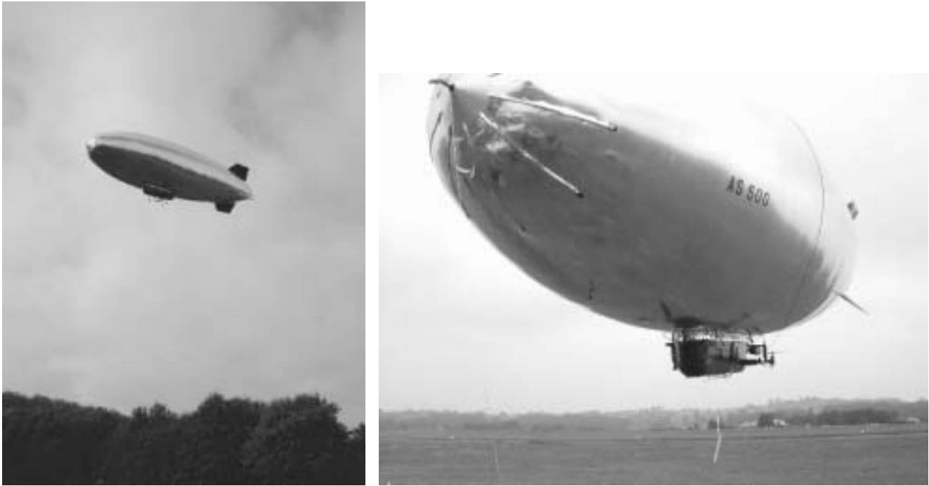
Fig. 1. Karma during its maiden flight in November 2001 (left, no on-board instrument were installed at that time), and during test flights in summer 2002 (right, the cameras and the Ethernet antenna are visible).
