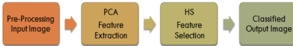
Figure 5. Block Diagram of HS-based Recognition System [13]
