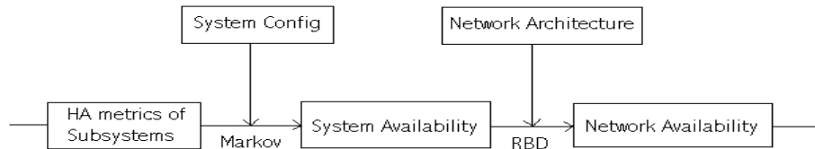
Figure 7.7. Modeling Flowchart for A Baseline Network
