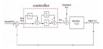
Fig.2 PD-PI controlled process.
