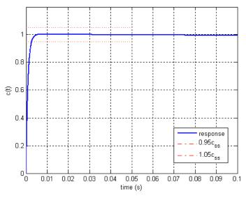
Fig.4 Step response of the PD-PI controlled second order process using the ITAE standard forms.
