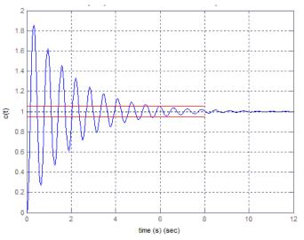
Fig.1 Step response of the uncontrolled process.
