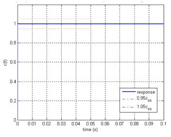
Fig.3 Step response of the PD-PI controlled second order process.
