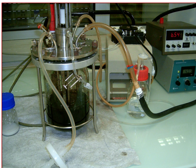
Fig 2.6 Bioconversion carried out for the bioconversion of glucose to gluconic acid, neutralised by 0.5M NaOH in 1.5L bioreactor.
