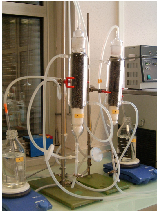
Fig 2.4. Production of spores by SSF in column fermentor.
