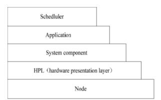
Figure 5 : The framework of TinyOS
