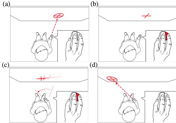
Figure 8: Dual-mode pointing. Ray-casting used for coarse-grained input (a). Activating precise mode via button press (b). Relative rotational movements control cursor movements (c). Switching back to coarse mode by releasing button (d). (Figure taken from [42].)
