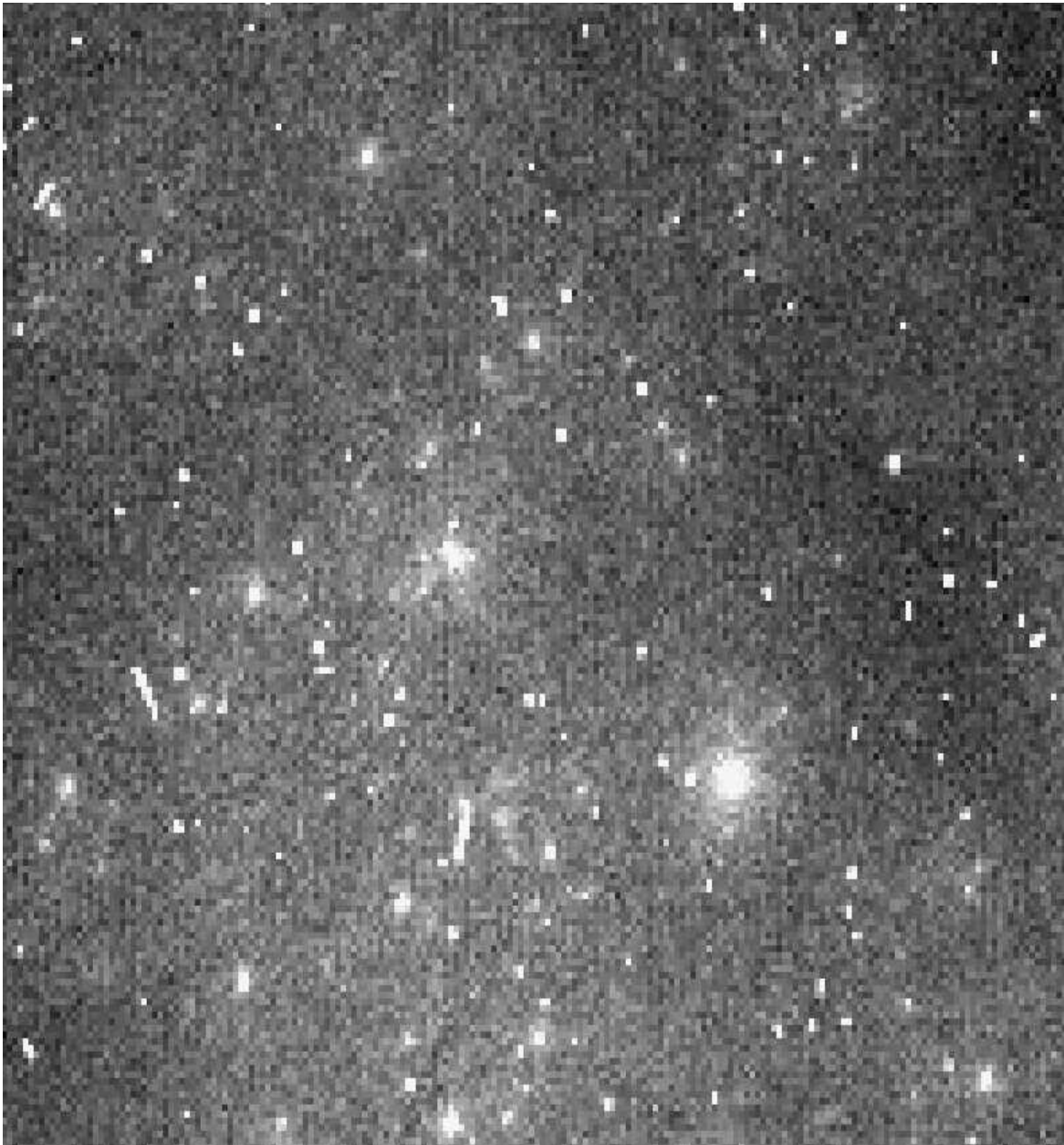
Figure 6.1: A portion of a 900 second CCD WF1 image of M81 taken through a yellow filter (F555W), containing stars, cosmic rays, and other sources of CCD and sky noise.
