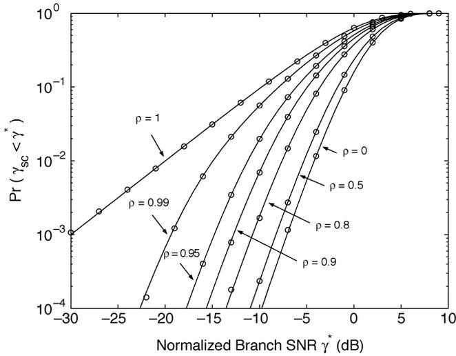
Fig. 2. Impact of fading correlation on the cdf of the SC output SNR in equally correlated Rayleigh fading;  $L = 4$ . Circles denote simulation points.
