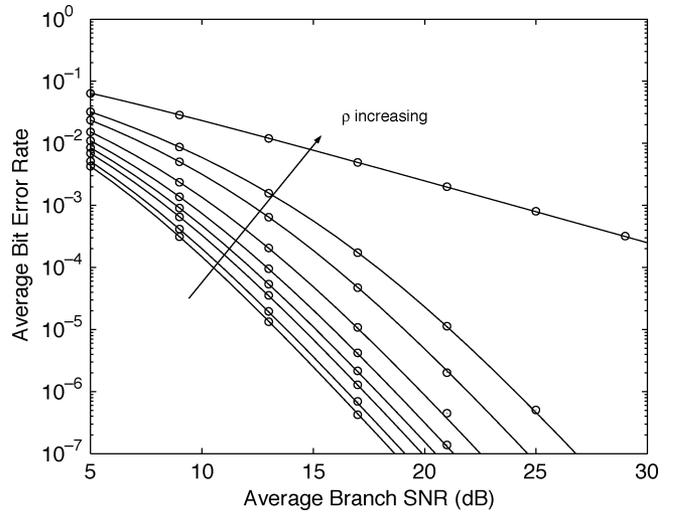
Fig. 5. Average BER of BPSK with four-branch SC in different equally correlated Rayleigh fading channels;  $\rho \in \{0, 0.3, 0.5, 0.6, 0.7, 0.8, 0.9, 0.95, 1\}$ . Circles denote simulation points.
