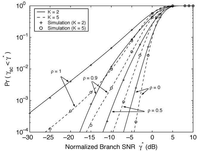
Fig. 3. Impact of fading correlation on the cdf of the SC output SNR in equally correlated Ricean fading;  $L = 4$ .
