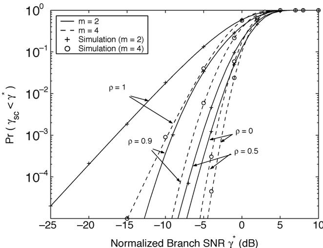
Fig. 4. Impact of fading correlation on the cdf of the SC output SNR in equally correlated Nakagami- $m$  fading;  $L = 4$ .
