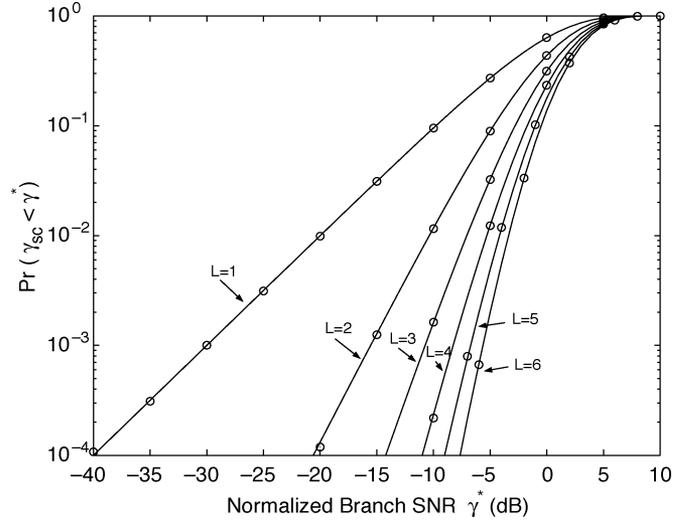
Fig. 1. CDF of the SC output SNR in equally correlated Rayleigh fading;  $\rho = 0.5$ . Circles denote simulation points.
