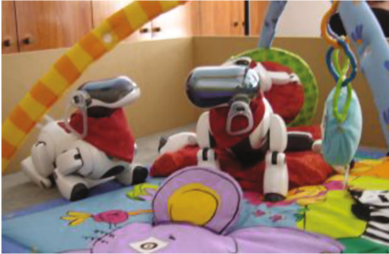
Fig. 1 The playground experiment setup involves a physical Sony AIBO robot which is put on a baby play mat with various toys, some of which affording learnable interactions, and an “adult robot” which is preprogrammed to imitate the vocalization of the learning robot when this later robot produces a vocalization while looking in the direction of the adult robot. The learning robot is equipped with a repertoire of innate parameterized sensorimotor primitives and learns driven by intrinsic motivation how to use and tune them to affect various aspects of its surrounding environment. Complex self-organized developmental trajectories emerge as a result of intrinsically motivated exploration, and the set of acquired skills and affordances increases along with time
