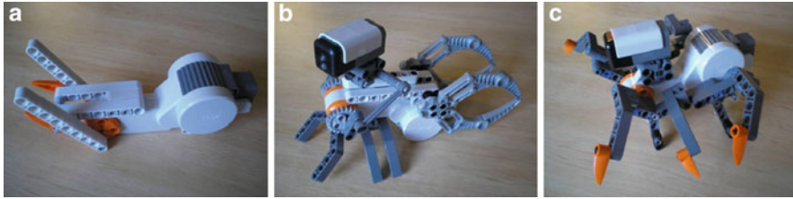
Fig. 6 Three Lego Mindstorms NXT robots (a) a snail with a single motor; (b) a bee with a motor and colour sensor; (c) an ant with a motor and accelerometer. Images from Merrick and Shafi (2009)
