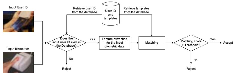
Fig. 1 Operation flow of a biometric verification system
