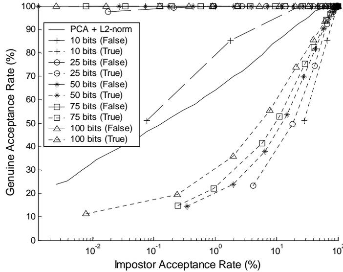
Fig. 4 ROC curves of various dimensions of FaceHash under different assumptions
