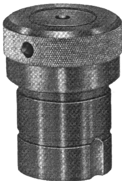
Fig. 1. Reaction vessels commonly used in solvothermal reactions. Top: loaded and sealed thick-wall Pyrex ampoules; Bottom: a Parr 23 ml acid digestion bomb.
