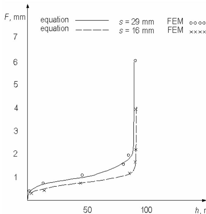
Figure 4. Numerical and experimental comparison the force  $F$  depending of punch motion  $h$
