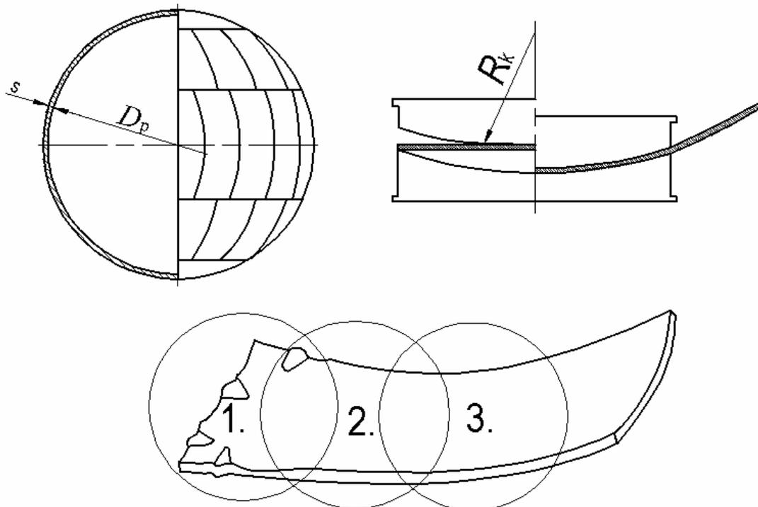
Figure 1. The bending of segment in tool
