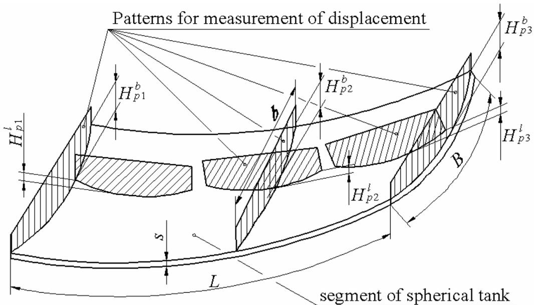
Figure 3: Pattern for displacement measurements
