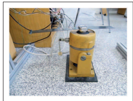
Figure 5. Steel sheet fixed to the shaker.
