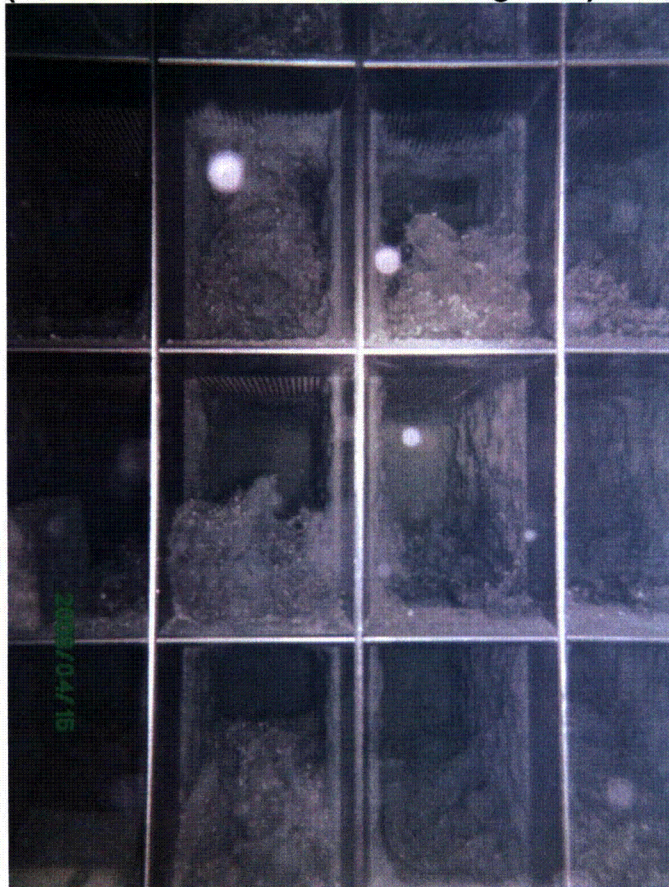
Figure 3-18: Test 2 Open Area with 100% Non-Chemical Debris (Underwater Photo Taken During Test)
