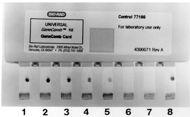
Figure 10. Results from use of a Gene Comb kit for detection of amplicons from templates of various concentrations of V. parahaemolyticus in haemolymph. Teeth 1 to 7, cell concentrations at 2 \times 10^7 , 10^6 , 10^5 , 10^4 , 10^3 , 10^2 , and 10^1 per ml; tooth 8 = control, with negative and positive control spots.
