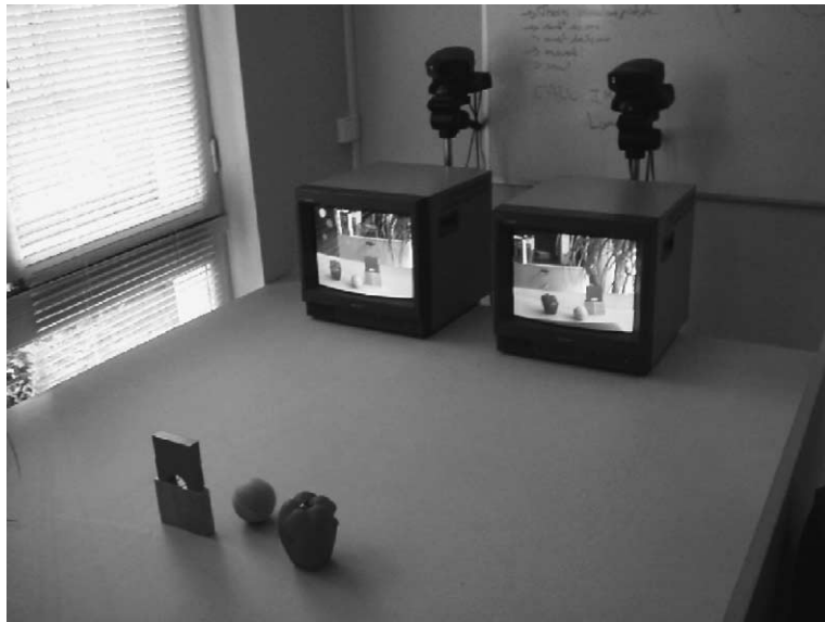
Fig. 1. Robotic installation used for the experiments reported in this paper. It consists of two steerable cameras capturing images of dynamic scenes. The captured images are shown on separate monitors.
