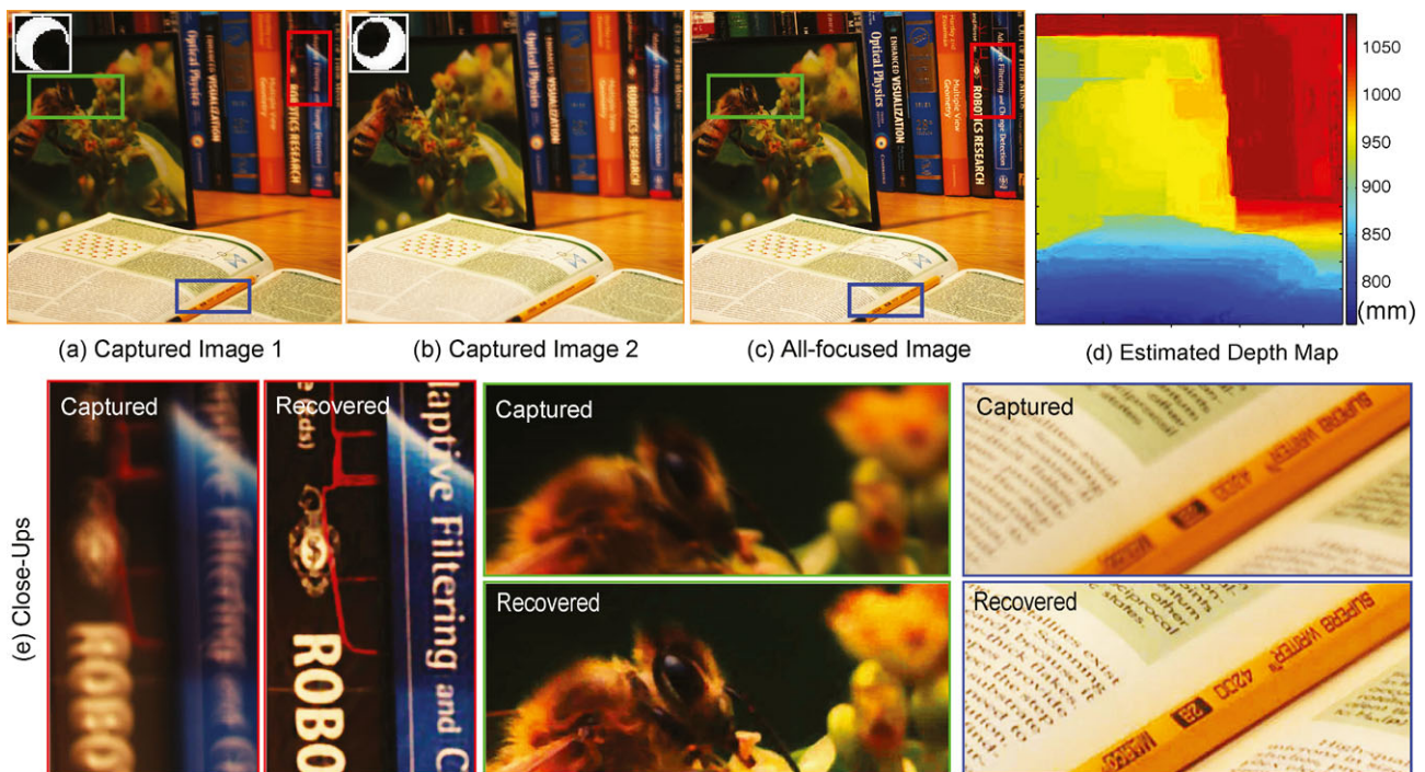
Fig. 2 (Color online) Depth from defocus and out-of-focus deblurring using a coded aperture pair. (a–b) Two captured images using the optimized coded aperture pair. The corresponding aperture patterns are shown at the top-left corner of each image. (c) The recovered all-focused image. (d) The estimated depth map. (e) Close-ups of four regions in the first captured image and the corresponding regions in the
