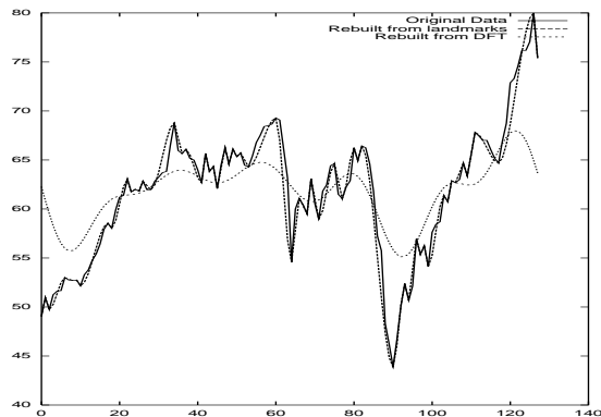
Figure 2. Cisco stock price from 6/1/1998 to 11/30/1998. The original time series, and the two time series reconstructed from first-order landmarks and from 4 DFT coefficients.
