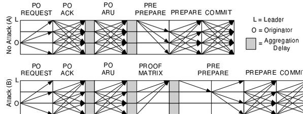
Figure 2: Common case operation of Prime ( $f = 1$ ). Part A shows the messages and protocol rounds when the leader is correct. Part B shows the delay added by a malicious leader that performs well enough to stay in power. The malicious leader ignores PO-ARU messages and sends its PRE-PREPARE to only one correct server.
