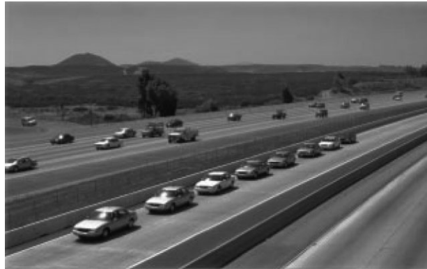
Figure 8. A platoon of cars driving down the San Diego freeway as part of the PATH project.
