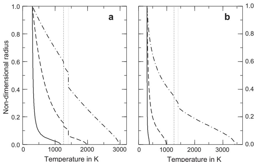
Fig. 2. Temperature as function of normalized radius for a planetesimal that has grown from an initial radius 5 km to its final radius 500 km over (a) 1 My and (b) 5 My immediately after the element synthesis. The exponent  $\beta$  in the growth rate law is 0 (dot-dashed line), 1 (dashed line), and 2 (solid line).
