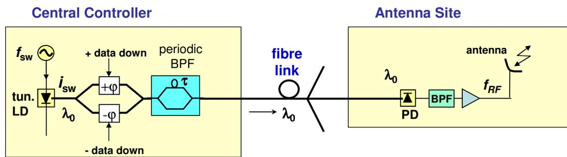
Fig. 2: Basic Optical Frequency Multiplication Scheme
