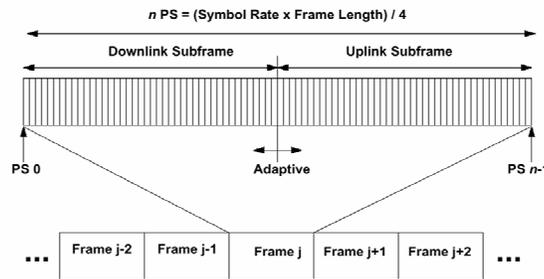
Fig. 7: IEEE 802.16 TDD frame structure
