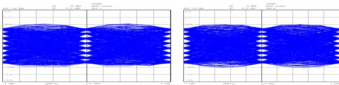
Fig. 5: I-eye and Q-eye diagrams of the 12Msymb/s 64-QAM signal (72Mbps) recovered at 17.8GHz after transmission over 4.4km of MMF
