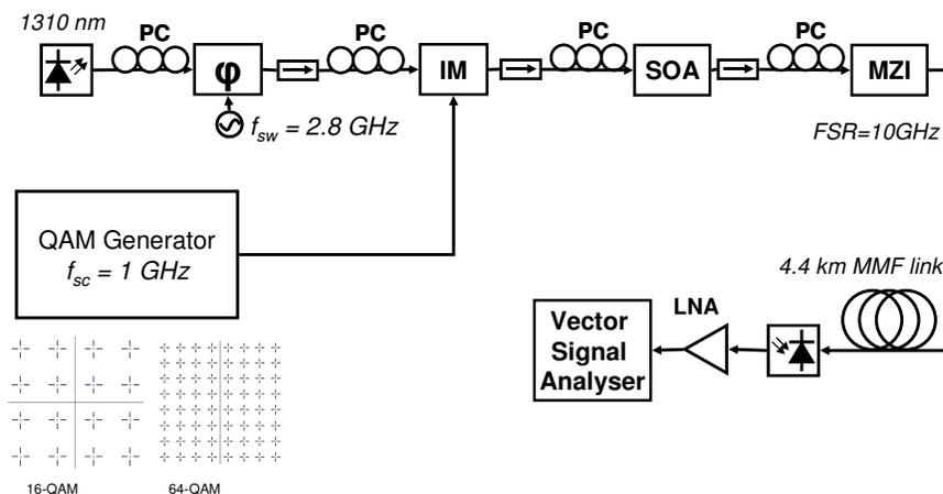
Fig. 3: Experimental setup; (PC: polarization controller)
