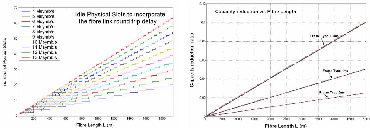
Fig. 8: IEEE 802.16 TDD frame capacity reduction for the accommodation of an optical fibre link between the CS and the AS
