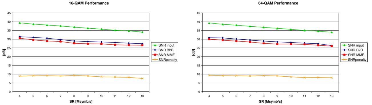
Fig. 6: Performance evaluation of the 16-QAM and 64-QAM signals obtained at 17.8GHz (SNR: signal-to-noise ratio; SR: symbol rate)
