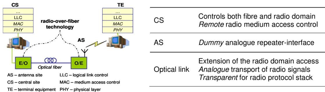
Fig. 1: Radio-over-fibre system approach
