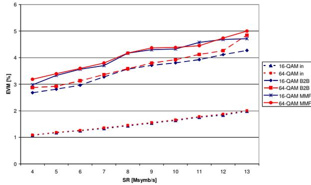
Fig. 4: Estimated EVM of the 16-QAM and 64-QAM signals obtained at 17.8GHz: input (at 1GHz), back-to-back and after 4.4km of MMF transmission (EVM: error vector magnitude; SR: symbol rate)
