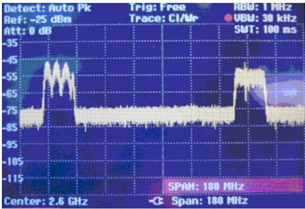
Fig. 11: Uplink (left) and downlink (right) spectrum on air.
