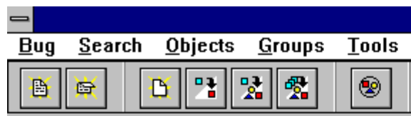
Figure 9-2: The main menu, and icon buttons for opening and closing access to specific project databases, create new bug reports, search for specific bugs in the database (three types of search), and for changing the role profile specified.
