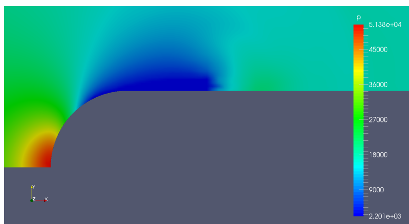
Figure 6-15: 2D cavitating head shape - water - \sigma = 0.4 , plot of pressure field
