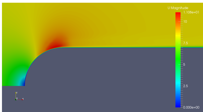
Figure 6-23: 2D cavitating head shape - propane - \sigma = 0.3 , plot of velocity field
