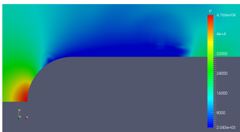
Figure 6-18: 2D cavitating head shape - water - \sigma = 0.3 , plot of pressure field
