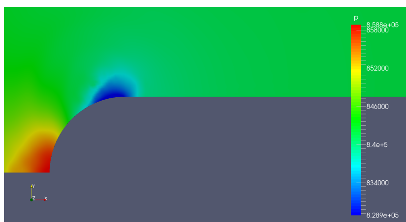
Figure 6-24: 2D cavitating head shape - propane - \sigma = 0.3 , plot of pressure field
