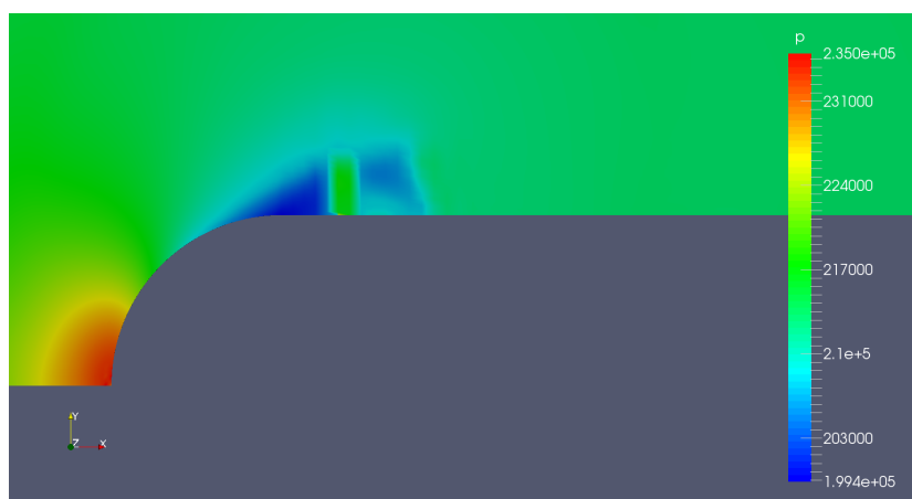
Figure 6-21: 2D cavitating head shape - butane - \sigma = 0.3 , plot of pressure field
