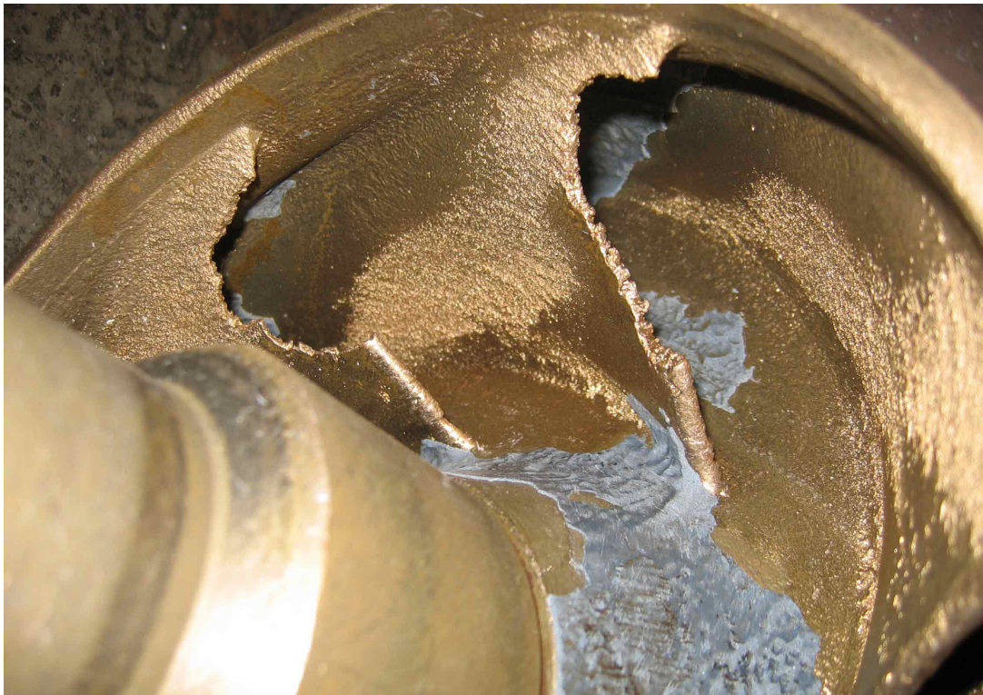
Figure 1-2: The resulting damage of continuous cavitation on a pump impeller [1]
