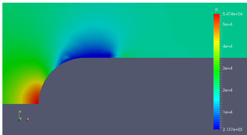
Figure 6-11: 2D cavitating head shape - water - \sigma = 0.5 , plot of velocity field
