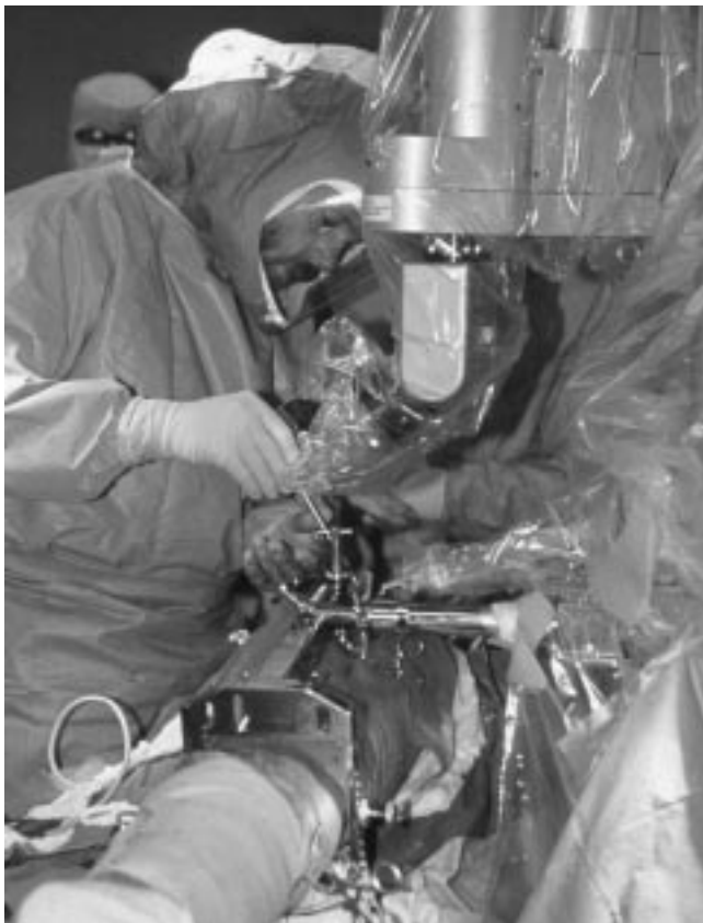
Fig. 1 'Robodoc' hip surgery robot
