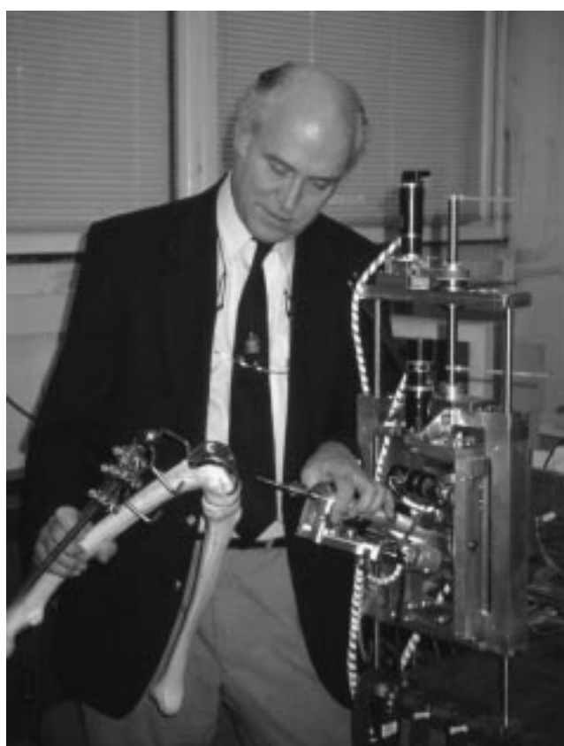
Fig. 5 Imperial College 'Acrobot' knee surgery robot with force-controlled handle
