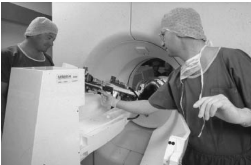
Fig. 4 'Minerva' neurosurgery robot in position, with the patient adjacent to a CT scanner
